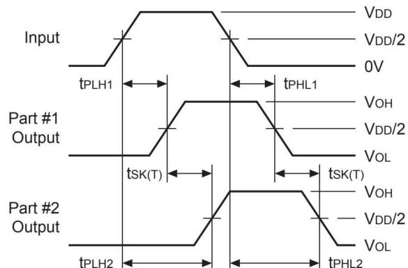
$$t_{SK(T)} = | t_{PLH2} - t_{PLH1} | \text{ or } | t_{PHL2} - t_{PHL1} |$$
