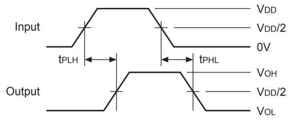
$$t_{sk(p)} = | t_{PLH} - t_{PHL} |$$
