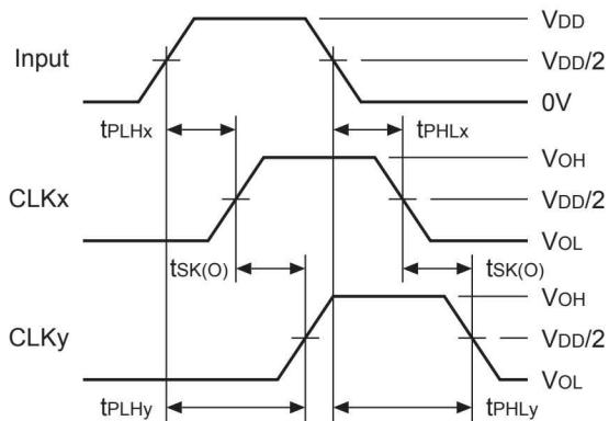
$$t_{SK(O)} = | t_{PLHy} - t_{PLHx} | \text{ or } | t_{PHLy} - t_{PHLx} |$$
