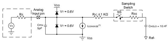
Legend: CPIN = Input Capacitance ILEAKAGE = Leakage Current at the pin due to various junctions = Interconnect Resistance Sampling Rs = Source Impedance Switch Rss VA = Analog Voltage  $(K\Omega)$ = Diode Forward Voltage Vт = Sampling Switch = Resistance of the Sampling Switch Rss 3 4 5 6 = Sample/Hold Capacitance CHOLD  $V_{DD}$ (V)
