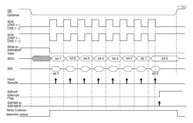
Figure 30-8. SPI Mode Waveform (Client Mode with CKE = 1)
