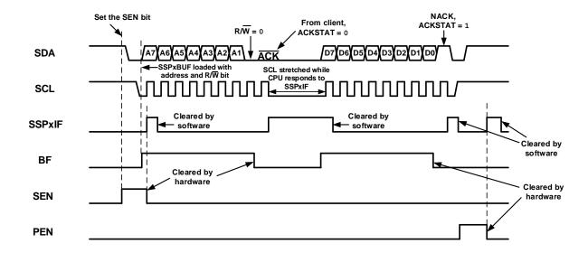
Figure 30-30. I<sup>2</sup>C Host Mode Waveform (Transmission, 10-Bit Address)
