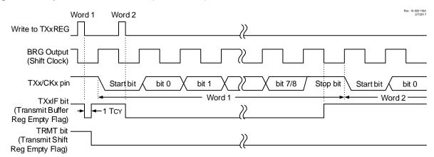
Figure 31-4. Asynchronous Transmission (Back-to-Back)
