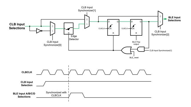
Figure 29-9. Edge Detector Operation when CLB Input Synchronizer[2:0] = '111'
