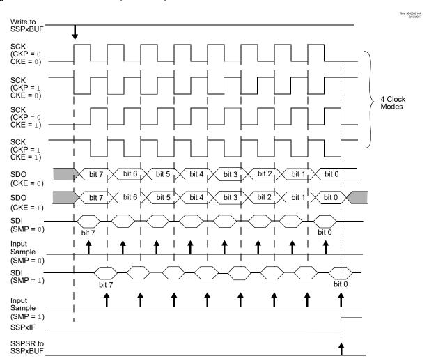
Figure 30-4. SPI Mode Waveform (Host Mode)
