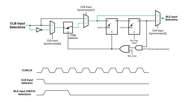
Figure 29-7. Edge Detector Operation when CLB Input Synchronizer[2:0] = '10X'
