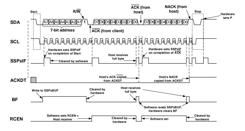
Figure 30-32. I<sup>2</sup>C Host Mode Waveform (Reception, 10-Bit Address)
