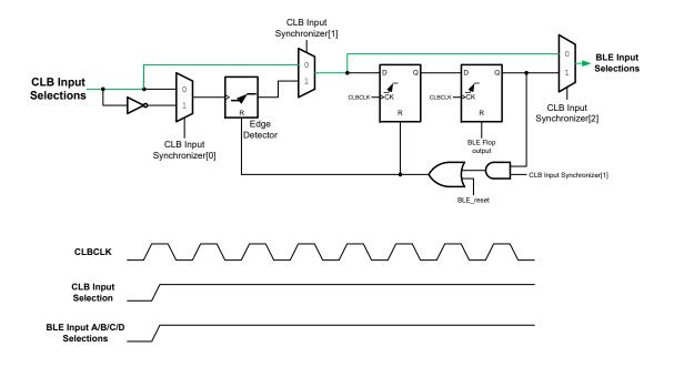
Figure 29-5. Edge Detector Operation when CLB Input Synchronizer[2:0] = '010'
