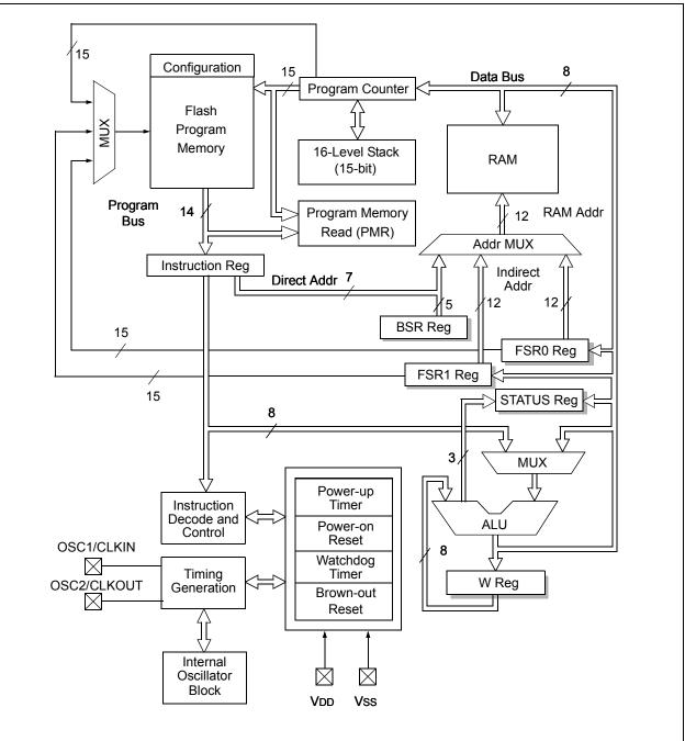
FIGURE 2-1: CORE BLOCK DIAGRAM
