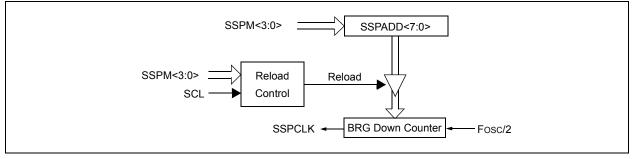
**Note:** Values of 0x00, 0x01 and 0x02 are not valid for SSPADD when used as a Baud Rate Generator for I<sup>2</sup>C. This is an implementation limitation.
