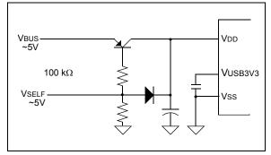
**Note:** Users should keep in mind the limits for devices drawing power from the USB. Refer to USB Specification 2.0, 7.2.3 for more information.
