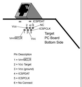
Another connector often found in use with the PICkit<sup>™</sup> programmers is a standard 6-pin header with 0.1 inch spacing. Refer to Figure 27-2.
