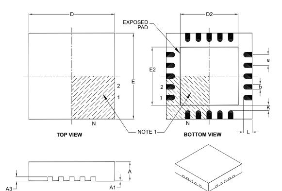
MILLIMETERS Units MIN NOM MAX **Dimension Limits** Number of Pins 20 Ν 0.50 BSC Pitch е **Overall Height** А 0.80 0.90 1.00 Standoff A1 0.00 0.02 0.05 **Contact Thickness** A3 0.20 REF 4.00 BSC Overall Width Е Exposed Pad Width E2 2.60 2.70 2.80 **Overall Length** 4.00 BSC D Exposed Pad Length D2 2.60 2.70 2.80 Contact Width 0.18 0.25 0.30 b 0.30 0.40 0.50 Contact Length L Contact-to-Exposed Pad Κ 0.20 \_ \_
