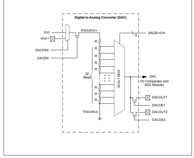
FIGURE 17-2: VOLTAGE REFERENCE OUTPUT BUFFER EXAMPLE
