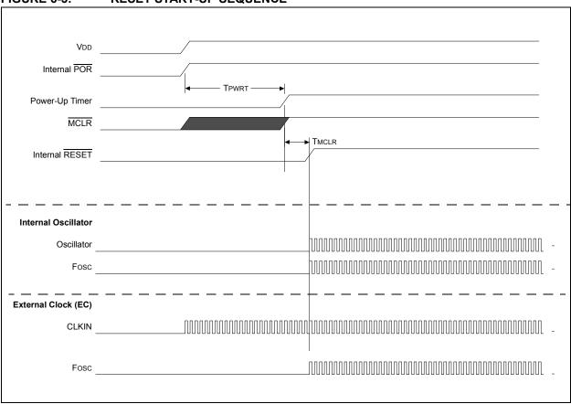
FIGURE 6-3: RESET START-UP SEQUENCE
