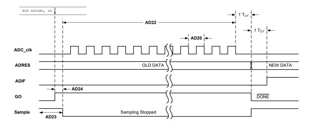
Figure 44-10. ADC Conversion Timing (ADC Clock from ADCRC)
