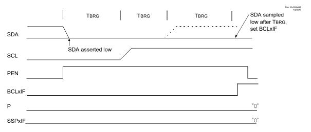
Figure 31-40. Bus Collision During a Stop Condition (Case 2)
