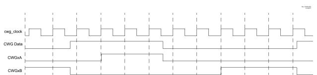
Figure 26-12. Dead-Band Operation, CWGxDBR = 0x01, CWGxDBF = 0x02
