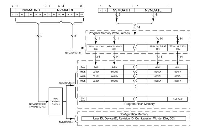
Figure 15-5. Program Flash Memory Write Sequence
