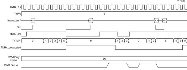
Note: 1. BSF and BCF represent Bit-Set File and Bit-Clear File instructions executed by the CPU to set or clear the ON bit of TxCON. CPU execution is asynchronous to the timer clock input.
