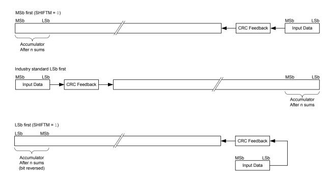
When the SHIFTM bit is not set, data will be shifted into the CRC, MSb first and the result will be big-endian. When the SHIFTM bit is set, data will be shifted into the accumulator in the reverse order (LSb first) and the result will be little-endian. The CRC module can be seeded with an initial value by setting the CRCOUT registers to the appropriate value before beginning the CRC process.
