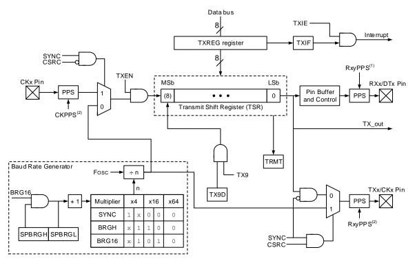
**Notes:** 1. In Synchronous mode, the DT output and RX input PPS selections will enable the same pin.
