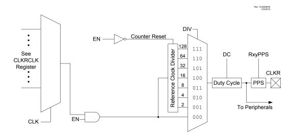
Figure 21-2. Clock Reference Timing
