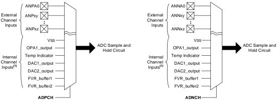
Note 1: The internal input channel selections vary. The inputs shown are all possible input selections. Please refer to the "ADC Positive Input Channel Selection" and "ADC Negative Input Channel Selection" tables for device-specific selection options.
