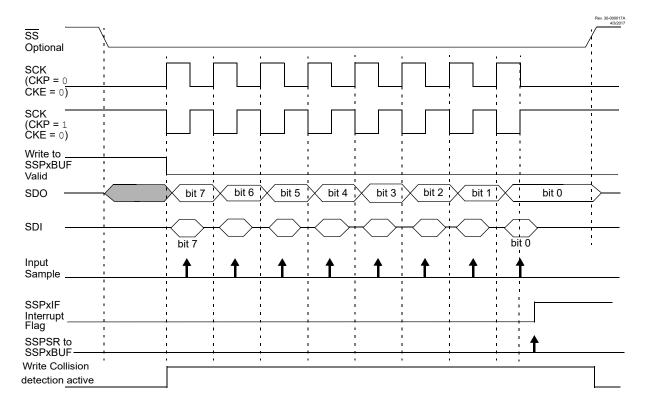
Figure 31-8. SPI Mode Waveform (Client Mode with CKE = 1)
