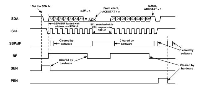
Figure 31-30. I<sup>2</sup>C Host Mode Waveform (Transmission, 10-Bit Address)
