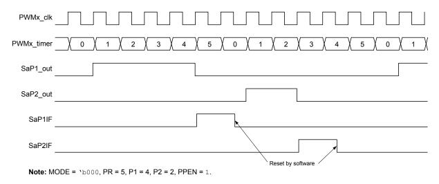
Figure 29-14. Right Aligned Push-Pull Mode Timing Diagram
