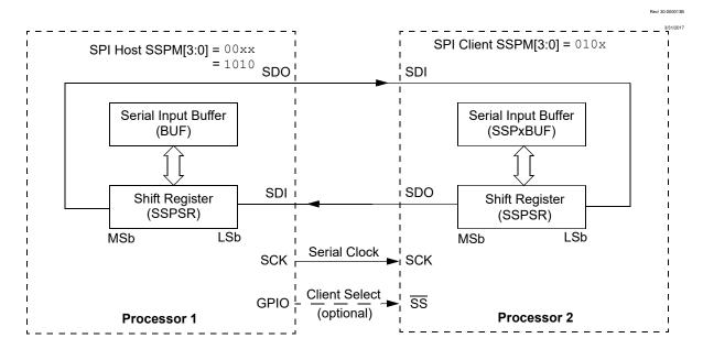
Data are shifted out of both shift registers on the programmed clock edge and are latched on the opposite edge of the clock.
