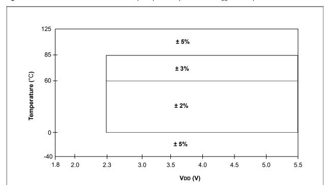
Figure 44-5. Precision Calibrated HFINTOSC Frequency Accuracy Over Device V<sub>DD</sub> and Temperature
