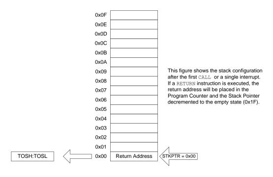
Figure 9-17. Accessing the Stack Example 3
