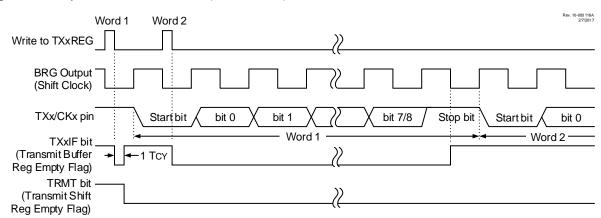
Figure 32-4. Asynchronous Transmission (Back-to-Back)
