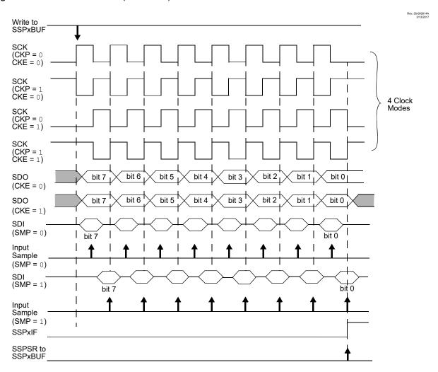
Figure 31-4. SPI Mode Waveform (Host Mode)
