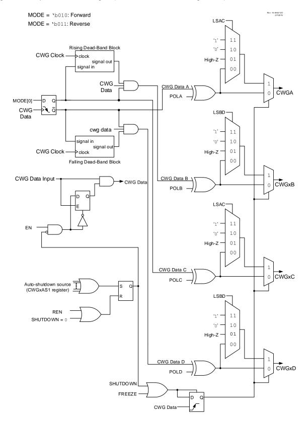
In Forward Full Bridge mode (MODE = <code>\b010</code>), CWGxA is driven to its Active state, CWGxB and CWGxC are driven to their Inactive state, and CWGxD is modulated by the input signal, as shown in Figure 26-7.
