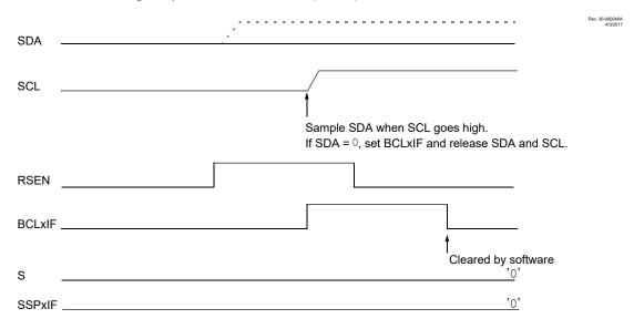
If SCL goes from high-to-low before the BRG times out and SDA has not already been asserted, a bus collision occurs. In this case, another host is attempting to transmit a data '1' during the Repeated Start condition (see Figure 31-38).
