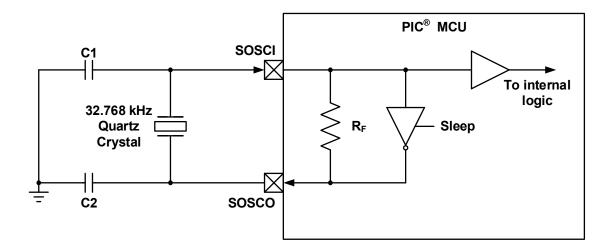
Figure 11-6. SOSC 32.768 kHz External Clock Operation
