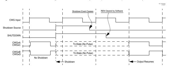
Figure 26-15. Shutdown Functionality, Auto-Restart Disabled (REN = 0, LSAC = 'b01, LSBD = 'b01)
