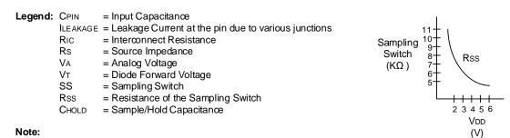
1. Refer to the "Electrical Specifications" chapter of the device data sheet for more details.
