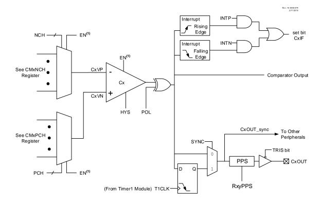
Figure 33-2. Comparator Module Simplified Block Diagram
