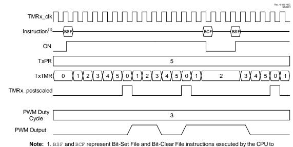
Figure 21-3. Software Gate Mode Timing Diagram (MODE = 'b00000)
