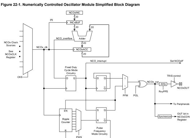
**Note 1:** The increment registers are double-buffered to allow for value changes to be made without first disabling the NCO module. The full increment value is loaded into the buffer registers on the second rising edge of the NCOx\_clk signal that occurs immediately after a write to the NCOxINCL register. The buffers are not user-accessible and are shown here for reference.
