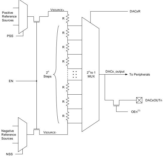
Note 1: The output enable bits are configured so that they act as a 'one-hot' system, meaning only one DAC output can be enabled at a time.
