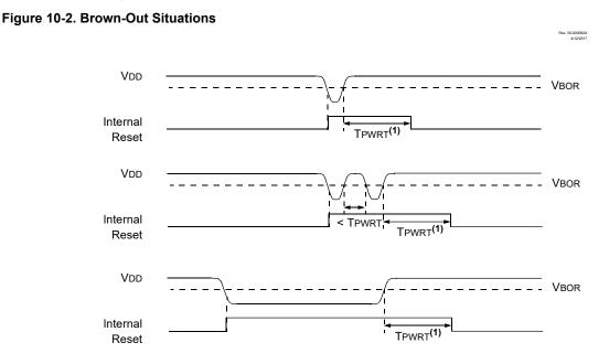
**Note:**  $T_{PWRT}$  delay when the PWRTS bits are enabled (<u>PWRTS</u> != 00).
