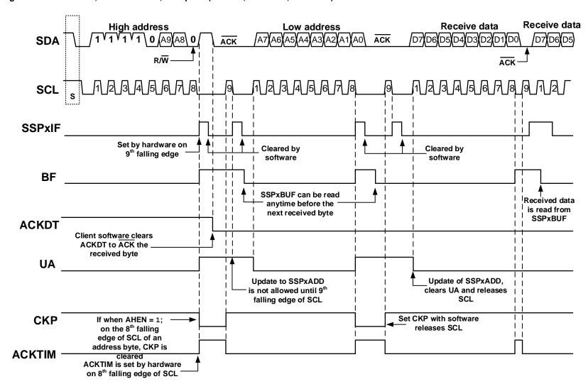
Figure 29-20. I<sup>2</sup>C Client, 10-Bit Address, Reception (SEN = 0, AHEN = 1, DHEN = 0)
