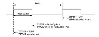
For a step-by-step procedure on how to set up this module for PWM operation, refer to 26.9. Setup for PWM Operation Using PWMx Output Pins.
