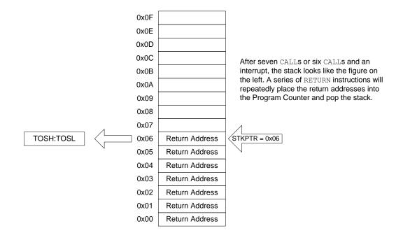
Figure 9-18. Accessing the Stack Example 4
