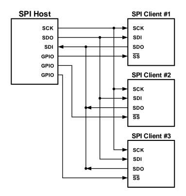
Transmissions involve two shift registers, eight bits in size: One in the host and one in the client. Data is always shifted out one bit at a time, with the Most Significant bit (MSb) shifted out first. At the same time, a new Least Significant bit (LSb) is shifted into the same register.
