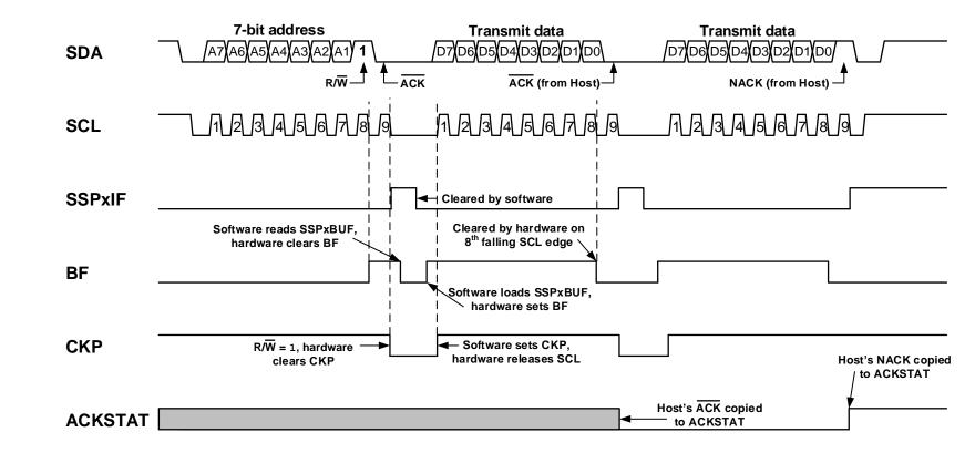
Figure 29-22. I<sup>2</sup>C Client, 7-Bit Address, Transmission (AHEN = 0)
