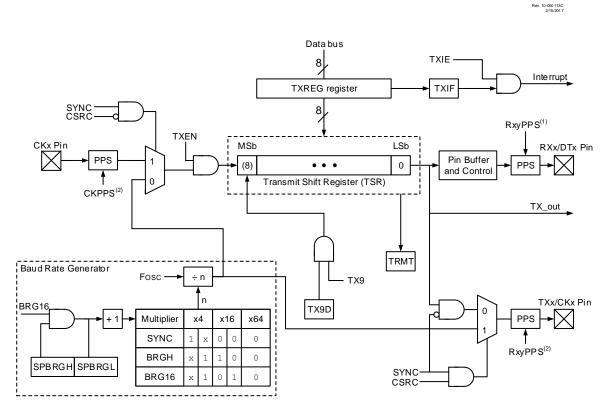
Notes: 1. In Synchronous mode, the DT output and RX input PPS selections will enable the same pin.
