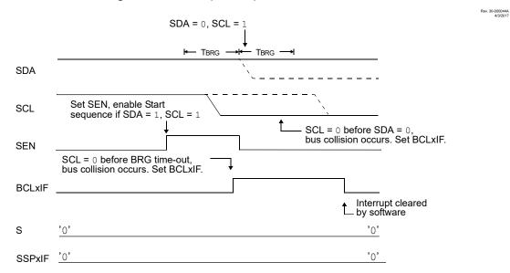
If the SDA pin is sampled low during this count, the BRG is reset and the SDA line is asserted early (see Figure 29-36). If, however, a '1' is sampled on the SDA pin, the SDA pin is asserted low at the end of the BRG count. The
