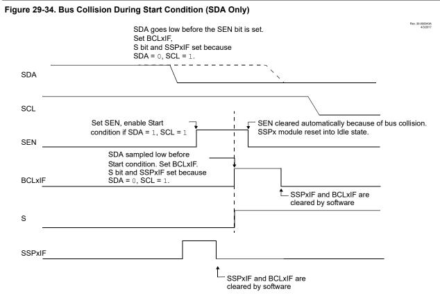
The Start condition begins with the SDA and SCL pins deasserted. When the SDA pin is sampled high, the Baud Rate Generator is loaded and counts down. If the SCL pin is sampled low while SDA is high, a bus collision occurs because it is assumed that another host is attempting to drive a data '1' during the Start condition.
