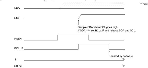
Figure 29-37. Bus Collision During a Repeated Start Condition (Case 1)
