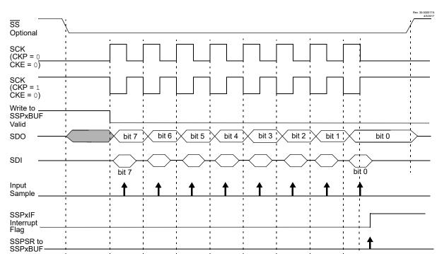
Figure 29-7. SPI Mode Waveform (Client Mode with CKE = 0)
