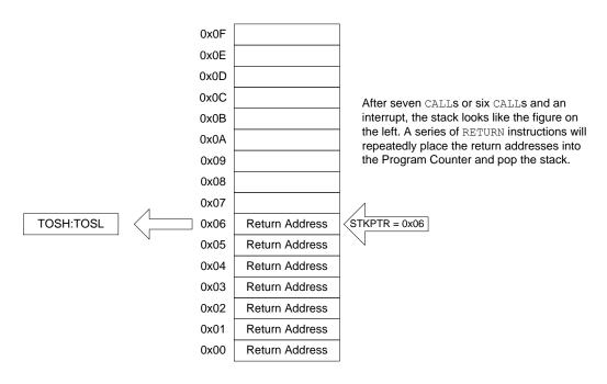
Figure 9-17. Accessing the Stack Example 4
