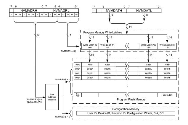
Figure 15-5. Program Flash Memory Write Sequence
