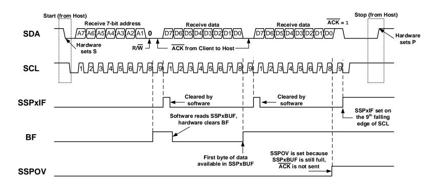
Figure 29-16. I<sup>2</sup>C Client, 7-Bit Address, Reception (SEN = 1, AHEN = 0, DHEN = 0)
