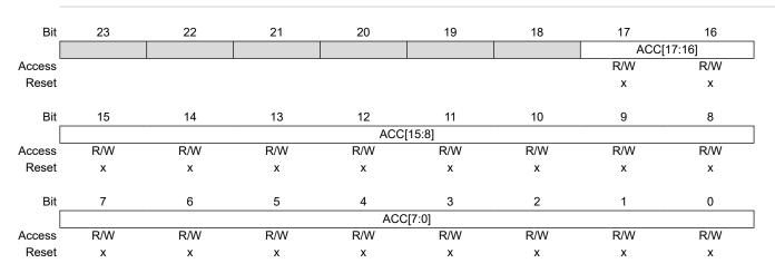
Bits 17:0 - ACC[17:0] ADC Accumulator - Signed two's complement
