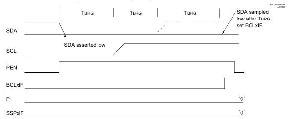
Figure 29-40. Bus Collision During a Stop Condition (Case 2)
