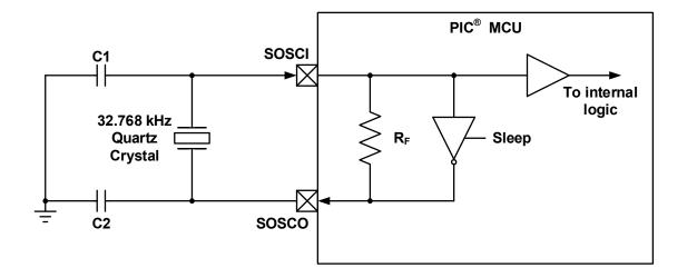
Figure 11-4. SOSC 32.768 kHz External Clock Operation
