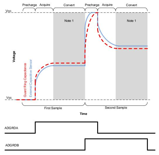
Figure 31-10. Differential CVD with Guard Ring Output Waveform
