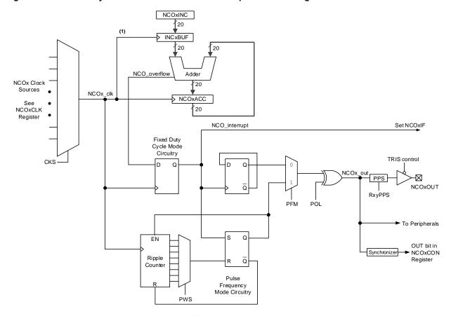
**Note 1:** The increment registers are double-buffered to allow for value changes to be made without first disabling the NCO module. The full increment value is loaded into the buffer registers on the second rising edge of the NCOx\_clk signal that occurs immediately after a write to the NCOxINCL register. The buffers are not user-accessible and are shown here for reference.
