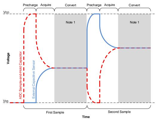
Figure 31-8. Differential CVD Measurement Waveform
