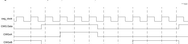
Figure 23-12. Dead-Band Operation, CWGxDBR = 0x01, CWGxDBF = 0x02
