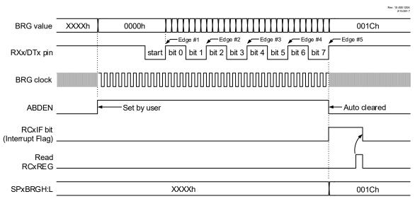
Figure 30-6. Automatic Baud Rate Calibration
