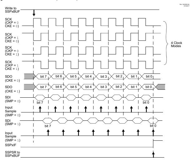
Figure 29-4. SPI Mode Waveform (Host Mode)
