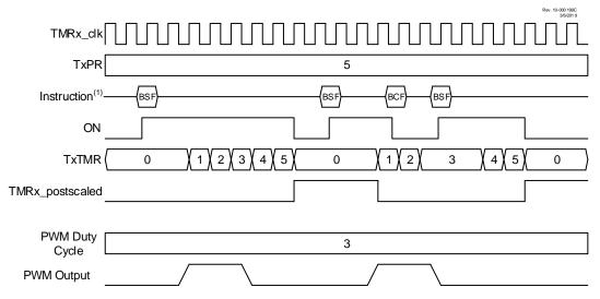
Note: 1. BSF and BCF represent Bit-Set File and Bit-Clear File instructions executed by the CPU to set or clear the ON bit of TxCON. CPU execution is asynchronous to the timer clock input.
