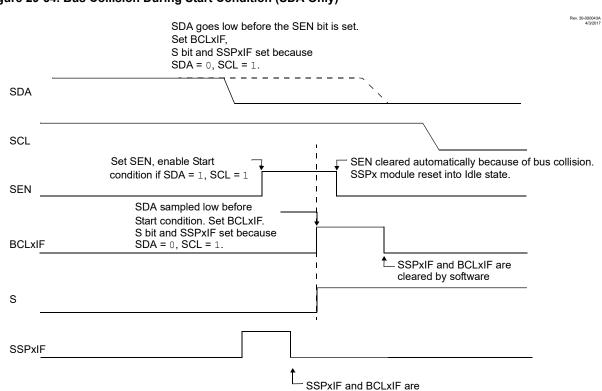
Figure 29-34. Bus Collision During Start Condition (SDA Only)
