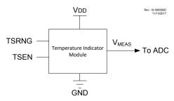
The output of the circuit is measured using the internal Analog-to-Digital Converter. A channel is reserved for the temperature circuit output. Refer to the "ADCC - Analog-to-Digital Converter with Computation Module" chapter for more details.
