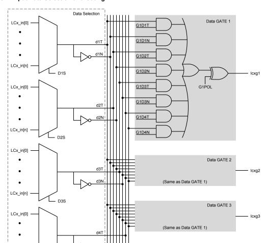
Figure 28-2. Input Data Selection and Gating
