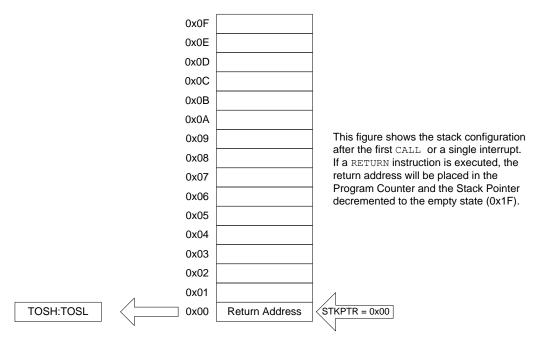
Figure 9-16. Accessing the Stack Example 3
