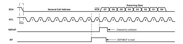
In 10-bit Address mode, the UA bit will not be set on the reception of the general call address. The client will prepare to receive the second byte as data, just as it would in 7-bit mode.
