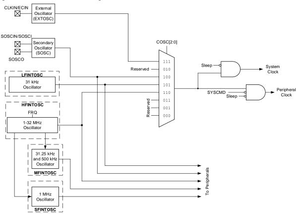
Figure 11-1. Clock Source Block Diagram
