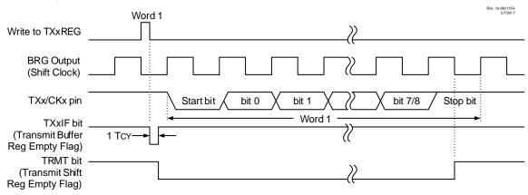
Figure 30-4. Asynchronous Transmission (Back-to-Back)
