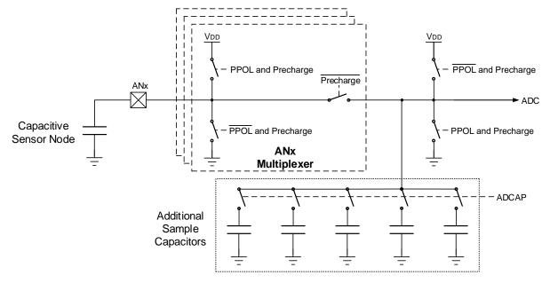
This is an example to configure ADC for CVD operation:
