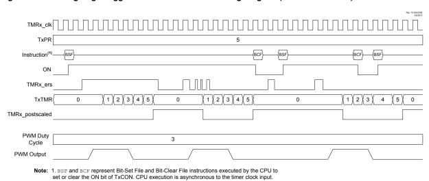
Figure 21-11. Rising Edge Triggered Monostable Mode Timing Diagram (MODE = vb10001)
