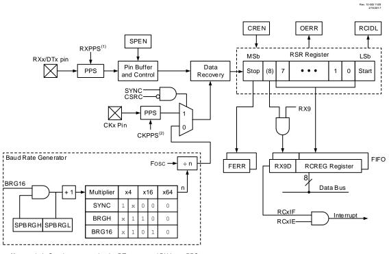
Figure 30-2. EUSART Receive Block Diagram
