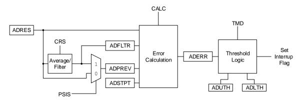
The operation of the ADC computational features is controlled by the MD bits.
