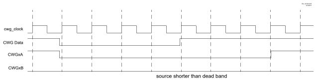
The CWGxDBF register value is double-buffered. When EN = 0, the buffer is loaded when CWGxDBF is written. When EN = 1, the buffer will be loaded at the rising edge following the first falling edge of the data input after the LD bit is set.
