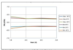
FIGURE 36-62: ADC 10-Bit Mode, Single-Ended INL, VDD = 3.0V, TAD = 4 μs, All devices
