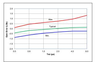
FIGURE 36-65: ADC 10-Bit Mode, Single-Ended Gain Error, VDD = 3.0V, VREF = 3.0V, -40°C to 85°C, All devices
