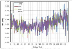
FIGURE 36-69: Typical DAC DNL Error, VDD = 3.0V, VREF = External 3V, All devices
