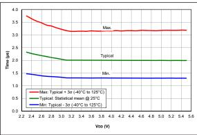
FIGURE 36-68: ADC RC Oscillator period, PIC16F18324/18344 Only
