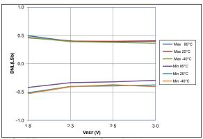
FIGURE 36-57: ADC 10-Bit Mode, Single-Ended DNL, VDD = 3.0V, TAD = 1 μs, All devices
