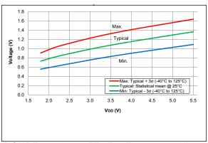
FIGURE 36-99: TTL Trip Thresholds, All devices
