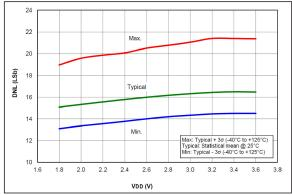
**FIGURE 36-73:** DAC INL Error, VDD = 3.0V, PIC16LF18324/18344 Only
