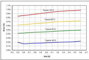
**FIGURE 36-92:** Typical FVR Voltage (1x), PIC16LF18324/18344 Only
