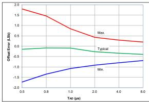
FIGURE 36-66: ADC 10-Bit Mode, Single-Ended Offset Error, VDD = 3.0V, VREF = 3.0V, -40°C to 85°C, All devices
