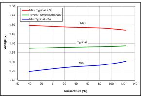
FIGURE 36-105: POR Release Voltage, All devices
