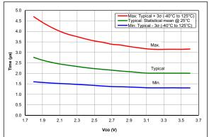
FIGURE 36-67: ADC RC Oscillator period, PIC16LF18324/18344 Only
