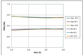
FIGURE 36-61: ADC 10-Bit Mode, Single-Ended DNL, VDD = 3.0V, TAD = 4 μs, All devices
