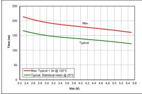
FIGURE 36-87: Comparator Response Time Falling edge, PIC16F18324/18344 Only
