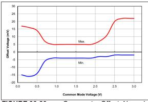
FIGURE 36-80: Comparator Offset, Normal Power Mode (CxSP = 1), VDD = 3.0V, Typical Measured Values from -40°C to 125°C, All devices
