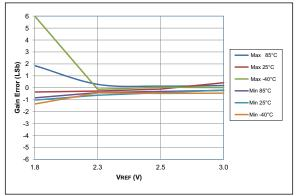
FIGURE 36-59: ADC 10-Bit Mode, Single-Ended Gain Error, VDD = 3.0V, TAD = 1 μs, All devices
