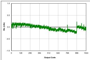
FIGURE 36-52: ADC 10-Bit Mode. Single-Ended INL, VDD = 3.0V, VREF = 3.0V,  $TAD = 1 \mu s$ , 25°C, All devices
