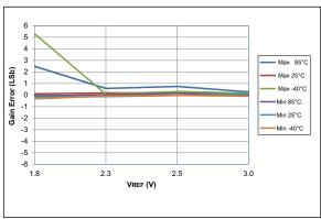
FIGURE 36-63: ADC 10-Bit Mode, Single-Ended Gain Error, VDD = 3.0V, TAD = 4 μs, All devices
