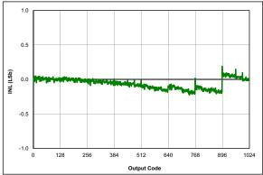
FIGURE 36-53: ADC 10-Bit Mode, Single-Ended INL, VDD = 3.0V, VREF = 3.0V,  $TAD = 4 \mu s$ , 25°C, All devices
