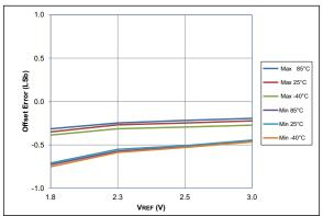
FIGURE 36-64: ADC 10-Bit Mode, Single-Ended Offset Error, VDD = 3.0V, TAD = 4 µs, All devices
