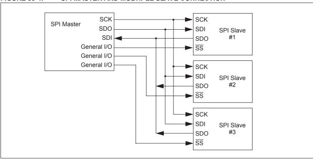
FIGURE 30-4: SPI MASTER AND MULTIPLE SLAVE CONNECTION
