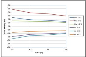
FIGURE 36-60: ADC 10-Bit Mode, Single-Ended Offset Error, VDD = 3.0V, TAD = 1 µs, All devices
