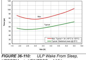
FIGURE 36-110: ULP Wake From Sleep, VREGPM = 1, HFINTOSC = 4 MHz, PIC16F18324/18344 Only
