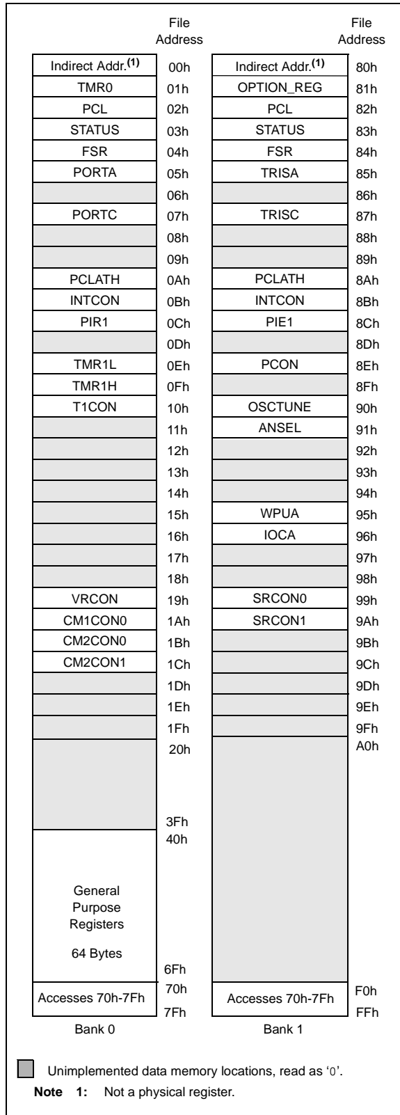
FIGURE 2-3: DATA MEMORY MAP OF THE PIC16F610/16HV610
