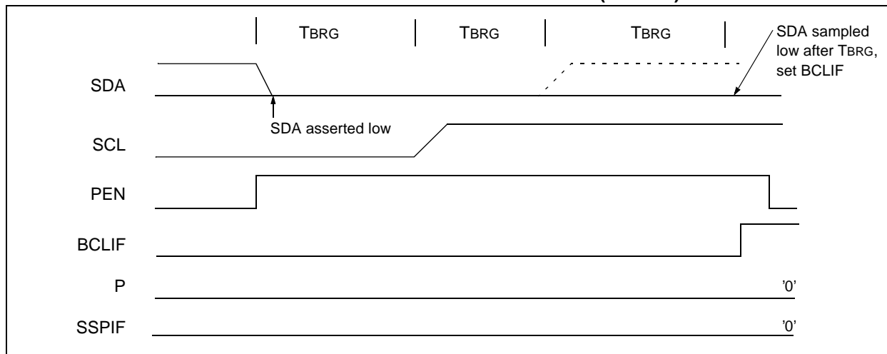
FIGURE 15-26: BUS COLLISION DURING A STOP CONDITION (CASE 1)
