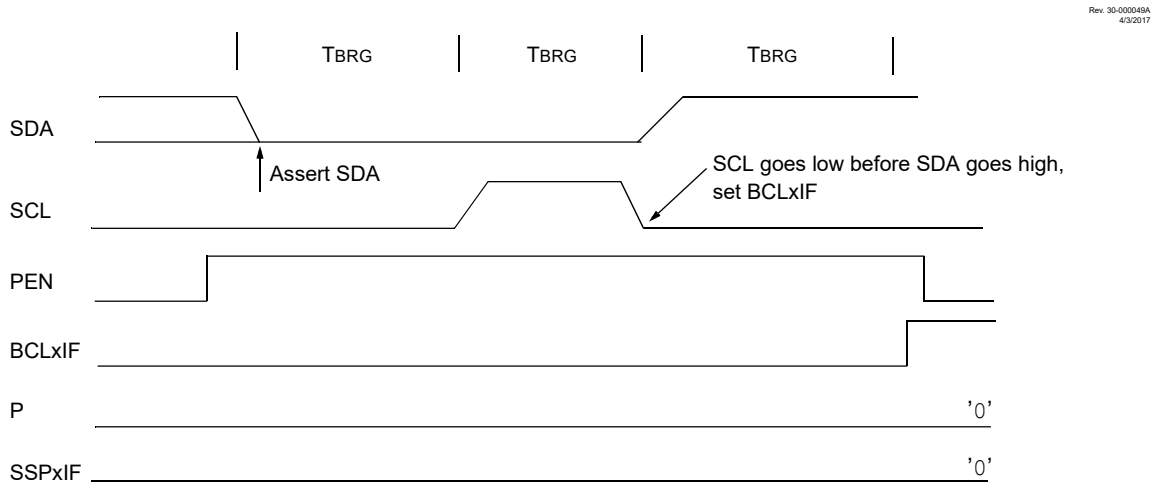
Figure 27-39. Bus Collision During a Stop Condition (Case 2)
