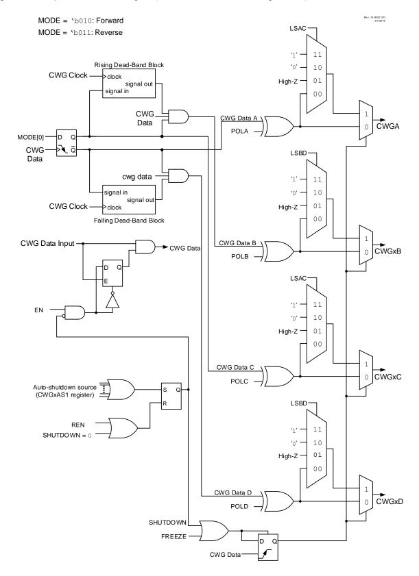
In Forward Full Bridge mode (MODE = 'b010), CWGxA is driven to its Active state, CWGxB and CWGxC are driven to their Inactive state, and CWGxD is modulated by the input signal, as shown in Figure 33-7.
