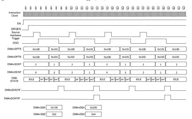
Figure 16-8. GPR-GPR Transactions with Hardware Triggers, SSTP, DSTP = 0
