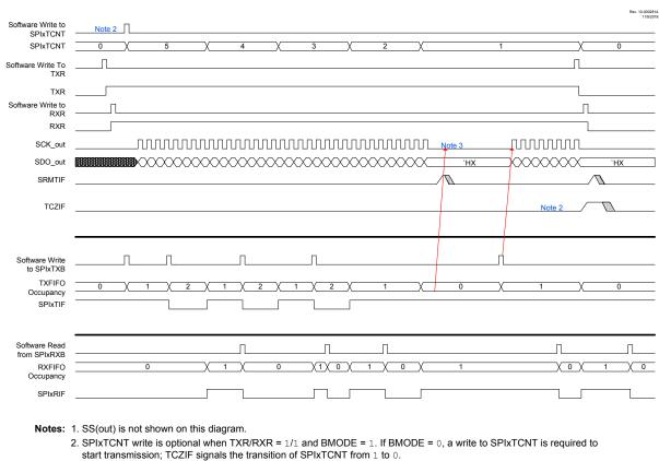
Figure 36-3. SPI Host Operation - Data Exchange, RXR = 1, TXR = 1
