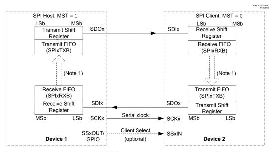
**Notes:** 1. In some modes, if the Transmit FIFO is empty, the most recently received byte of data will be transmitted.
