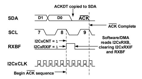
Figure 37-35. Not Acknowledge (NACK) Sequence Timing
