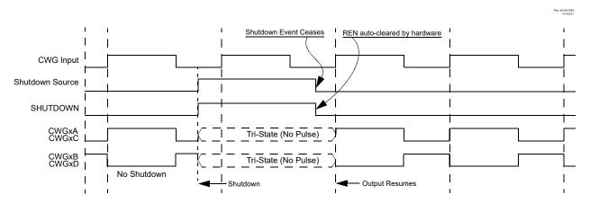
Figure 33-16. Shutdown Functionality, Auto-Restart Enabled (REN = 1, LSAC = 'b01, LSBD = 'b01)
