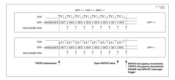
Figure 36-10. Clocking Detail - Host Mode, CKE = 1, SMP = 0
