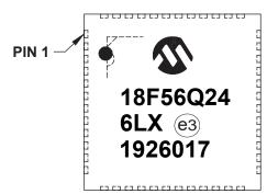
48-Lead TQFP (7x7x1 mm)
