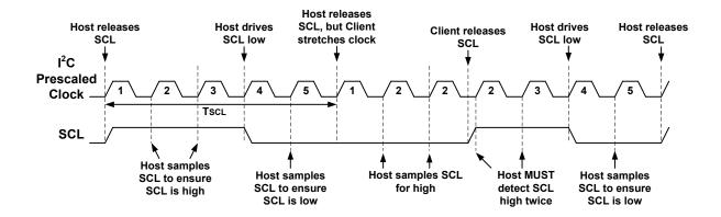
When FME = 1, one SCL period ( $T_{SCL}$ ) is equal to four clock periods of the prescaled I2CxCLK source. In other words, the prescaled I2CxCLK source is divided by four. Using the example from above, if the HFINTOSC (4 MHz) clock source is selected, I2CxBAUD is loaded with a value of '7', and FME = 1, the actual SCL frequency is 125 kHz (see the equation below).
