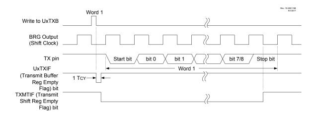
Figure 35-4. UART Asynchronous Transmission (Back-to-Back)
