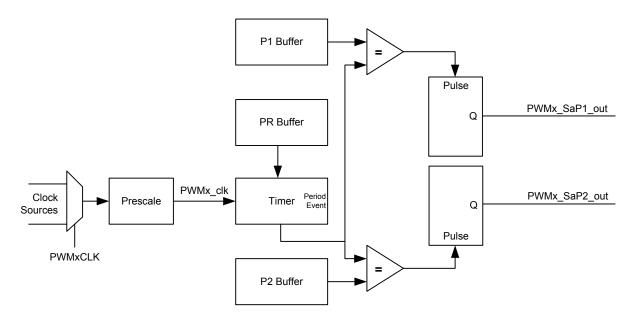
Figure 32-10. Pulsed Compare Timing Diagram
