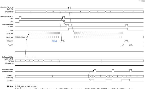
Figure 36-5. SPI Host Operation - Command+Read Data, TXR = 0, RXR = 1
