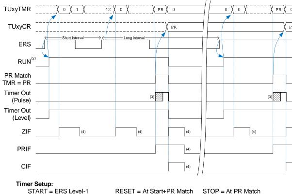
Figure 29-11. Reset at Level Start and Stop at PR Match
