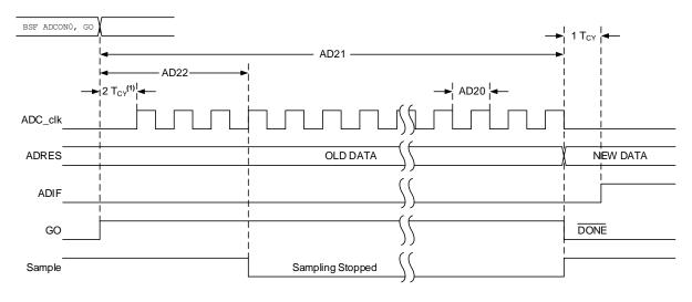
Note 1: If the ADC clock source is selected as ADCRC, a time of 1 TCY is added before the ADC clock starts. This allows the SLEEP instruction to be executed, if any.
