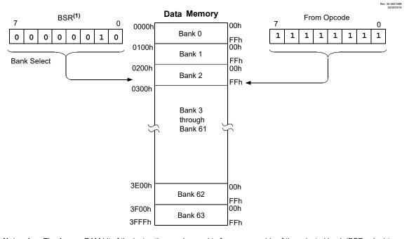
Note 1: The Access RAM bit of the instruction can be used to force an override of the selected bank (BSR value) to the registers of the Access Bank.
