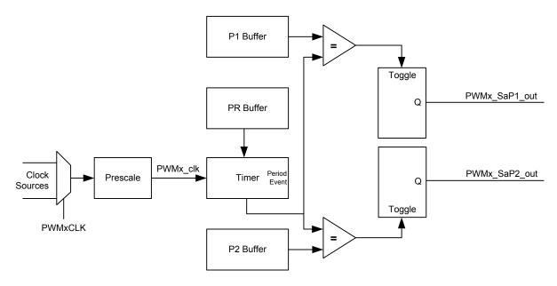
Figure 32-12. Toggled Compare Timing Diagram
