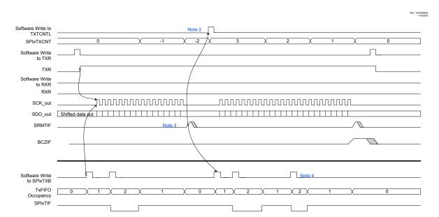
**Figure 36-4.** SPI Host Operation - Command+Write Data, TXR = 1, RXR = 0
