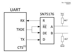
Note 1: Configure UxCTSPPS to an unimplemented input such as RD0. (e.g. UxCTSPPS = 0x18)
