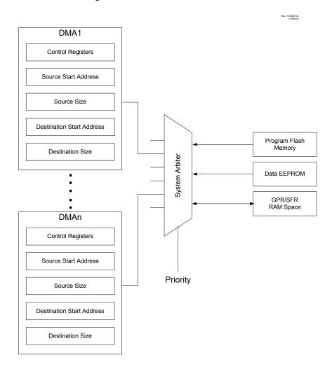
Depending on the priority of the DMA with respect to CPU execution (refer to the "Memory Access Scheme" section in the "PIC18 CPU" chapter for more information), the DMA Controller can move data through two methods:
