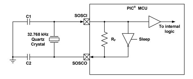
Figure 12-6. SOSC 32.768 kHz External Clock Operation
