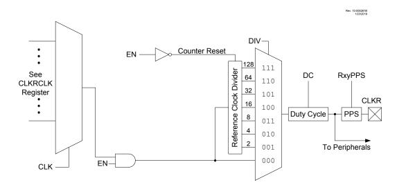
Figure 25-2. Clock Reference Timing
