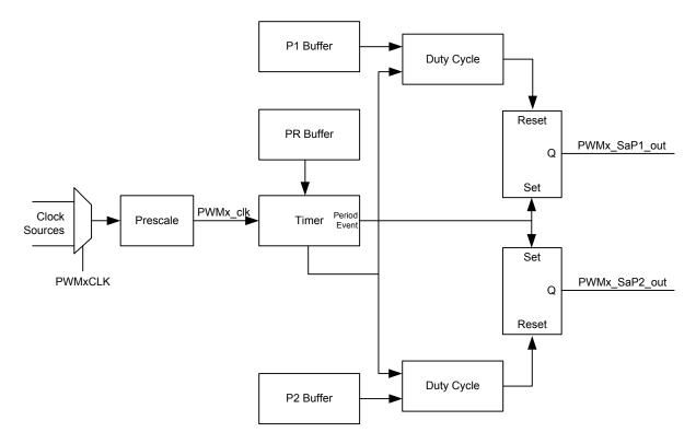
Figure 32-2. Left-Aligned Timing Diagram
