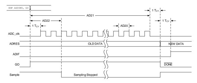
Figure 48-10. ADC Conversion Timing (ADC Clock from ADCRC)
