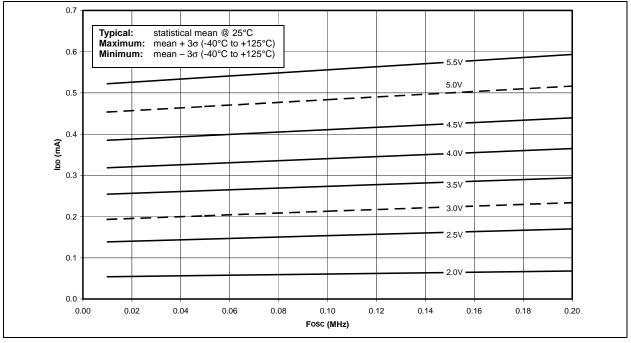
FIGURE 27-3: MAXIMUM IDD vs. FOSC OVER VDD PRI\_RUN, EC MODE, -40°C TO +125°C
