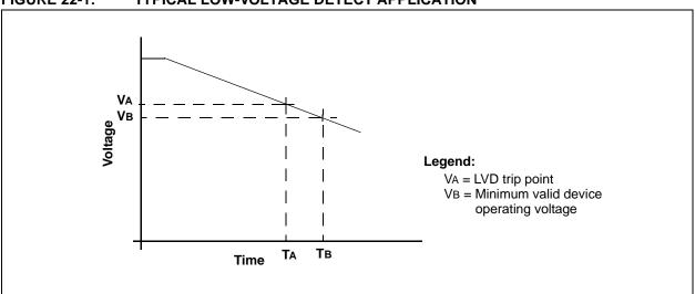
FIGURE 22-1: TYPICAL LOW-VOLTAGE DETECT APPLICATION
