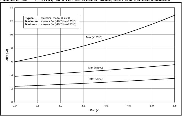
FIGURE 27-31:  $\triangle$ IPD LVD vs. VDD SLEEP MODE, LVD = 2.00V-2.12V
