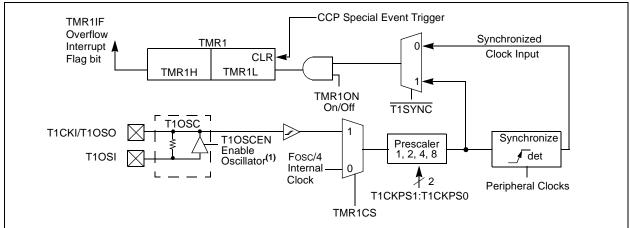
Note 1: When enable bit T1OSCEN is cleared, the inverter and feedback resistor are turned off. This eliminates power drain.
