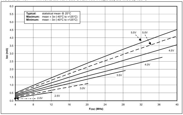
FIGURE 27-14: MAXIMUM IDD vs. FOSC OVER VDD PRI\_IDLE, EC MODE, -40°C TO +125°C
