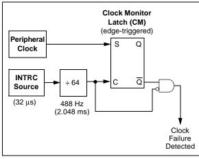
Clock failure is tested on the falling edge of the sample clock. If a sample clock falling edge occurs while CM is still set, a clock failure has been detected (Figure 23-4). This causes the following:
