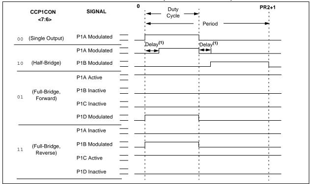
FIGURE 16-3: PWM OUTPUT RELATIONSHIPS (ACTIVE-LOW STATE)
