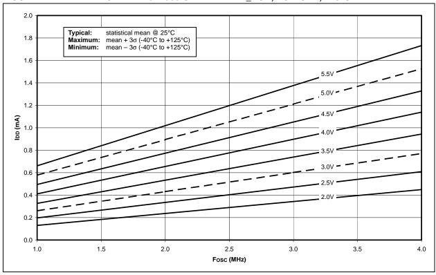
FIGURE 27-5: MAXIMUM IDD vs. Fosc OVER VDD PRI\_RUN, EC MODE, -40°C TO +125°C
