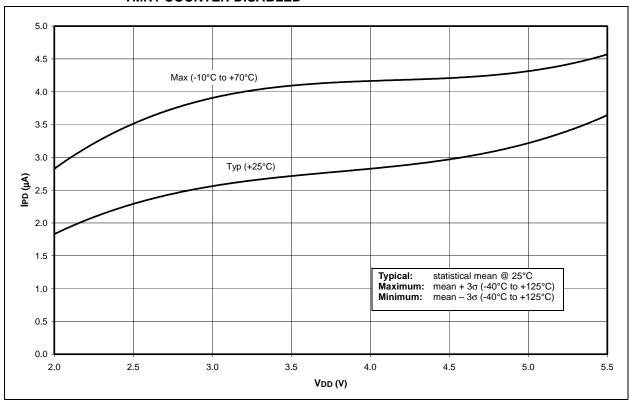
FIGURE 27-29:  $\triangle$ IPD FSCM vs. VDD OVER TEMPERATURE PRI\_IDLE, EC OSCILLATOR AT 32 kHz, -40°C TO +125°C
