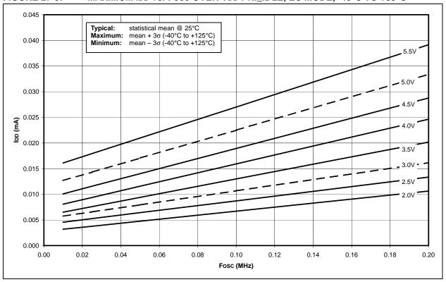
FIGURE 27-10: MAXIMUM IDD vs. FOSC OVER VDD PRI\_IDLE, EC MODE, -40°C TO +125°C
