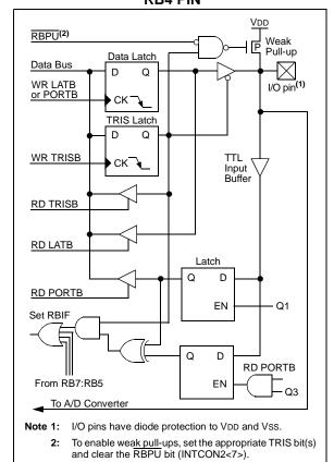
To enable weak pull-ups, set the appropriate TRIS bit(s) and clear the RBPU bit (INTCON2<7>).
