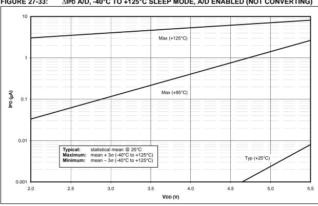
FIGURE 27-33: △IPD A/D, -40°C TO +125°C SLEEP MODE, A/D ENABLED (NOT CONVERTING)
