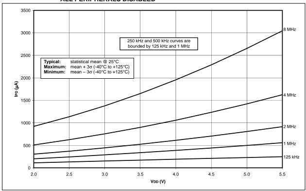
FIGURE 27-17: TYPICAL AND MAXIMUM IPD vs. VDD (-40°C TO +125°C), 31.25 kHz RC\_RUN, ALL PERIPHERALS DISABLED
