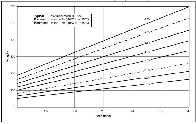
FIGURE 27-13: TYPICAL IDD vs. FOSC OVER VDD PRI\_IDLE, EC MODE, +25°C
