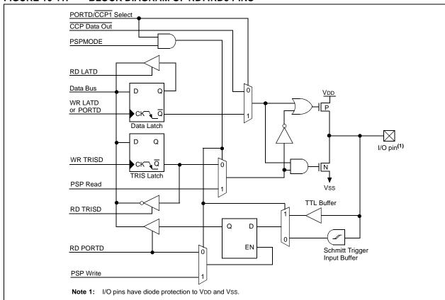
FIGURE 10-12: BLOCK DIAGRAM OF RD4:RD0 PINS
