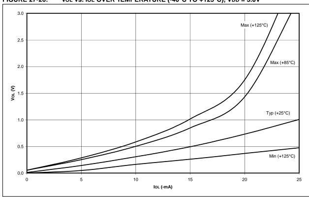
FIGURE 27-27: Vol vs. Iol OVER TEMPERATURE (-40°C TO +125°C), VDD = 5.0V
