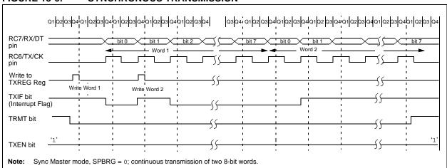
FIGURE 18-7: SYNCHRONOUS TRANSMISSION (THROUGH TXEN)
