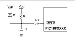
Note 1: External Power-on Reset circuit is required only if the VDD power-up slope is too slow. The diode D helps discharge the capacitor quickly when VDD powers down.
