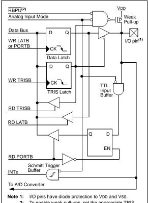
FIGURE 10-8: BLOCK DIAGRAM OF RB4 PIN
