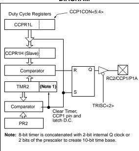
A PWM output (Figure 15-4) has a time base (*period*) and a time that the output is high (*duty cycle*). The frequency of the PWM is the inverse of the period (1/period).
