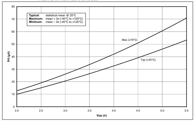
FIGURE 27-22: IPD SEC\_IDLE, -10°C TO +70°C 32.768 kHz 2 X 22 pF, ALL PERIPHERALS DISABLED
