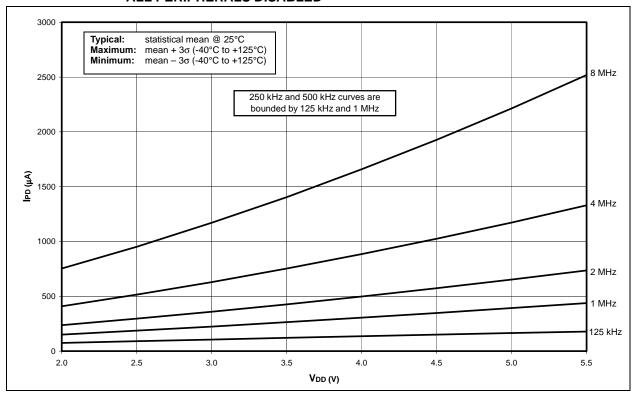
FIGURE 27-16: MAXIMUM IPD vs. VDD (-40°C TO +125°C), 125 kHz TO 8 MHz RC\_RUN, ALL PERIPHERALS DISABLED
