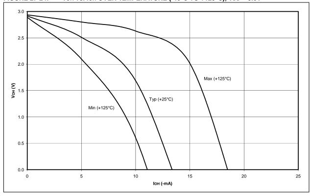
FIGURE 27-25: Voh vs. Ioh OVER TEMPERATURE (-40°C TO +125°C), VDD = 5.0V
