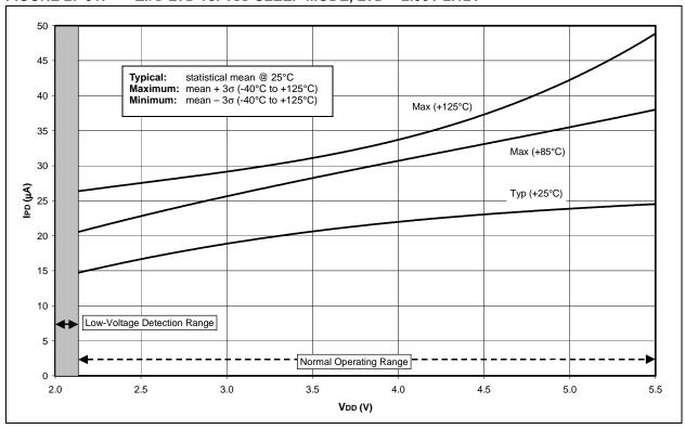
FIGURE 27-32:  $\triangle$ IPD BOR vs. VDD, -40°C TO +125°C SLEEP MODE, BOR ENABLED AT 2.00V-2.16V
