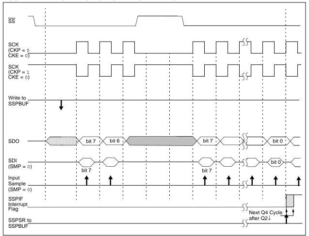
FIGURE 17-5: SPI MODE WAVEFORM (SLAVE MODE WITH CKE = 0)
