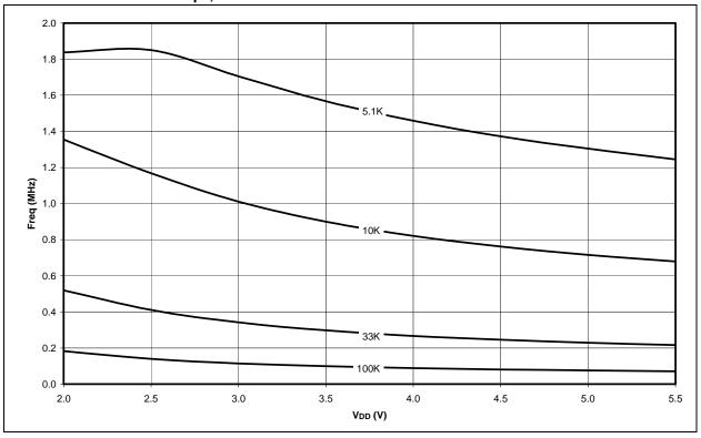
FIGURE 27-36: AVERAGE FOSC vs. VDD FOR VARIOUS R'S EXTERNAL RC MODE, C = 300 pF, TEMPERATURE = +25°C
