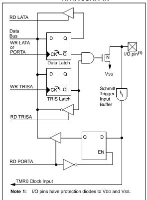
FIGURE 10-5: BLOCK DIAGRAM OF RA7 PIN
