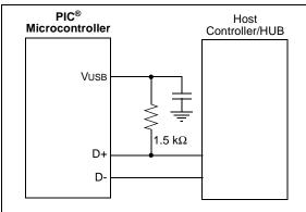
Note: The above setting shows a typical connection for a full-speed configuration using an on-chip regulator and an external pull-up resistor.
