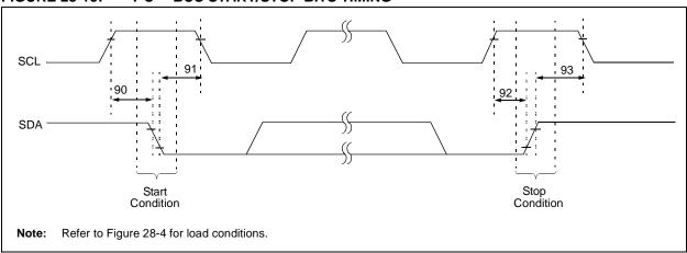
TABLE 28-19: I<sup>2</sup>C™ BUS START/STOP BITS REQUIREMENTS (SLAVE MODE)
