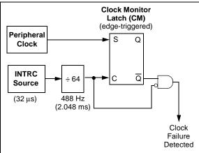
Clock failure is tested for on the falling edge of the sample clock. If a sample clock falling edge occurs while CM is still set, a clock failure has been detected (Figure 25-4). This causes the following:
