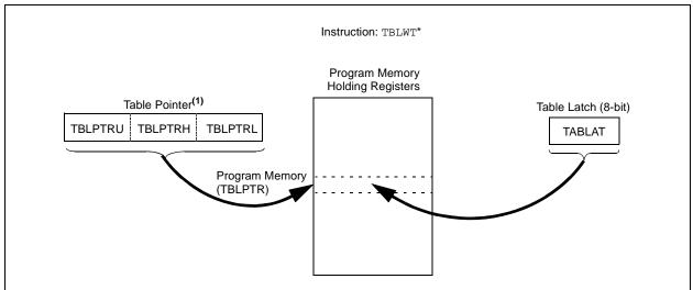
Note 1: Table Pointer actually points to one of 32 holding registers, the address of which is determined by TBLPTRL<4:0>. The process for physically writing data to the program memory array is discussed in Section 6.5 "Writing to Flash Program Memory".
