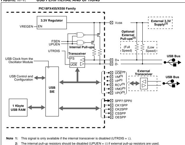
3: Do not enable the internal regulator when using an external 3.3V supply.
