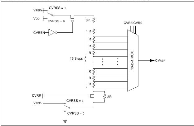
FIGURE 23-1: COMPARATOR VOLTAGE REFERENCE BLOCK DIAGRAM
