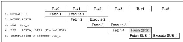
**Note:** All instructions are single cycle, except for any program branches. These take two cycles since the fetch instruction is "flushed" from the pipeline while the new instruction is being fetched and then executed.
