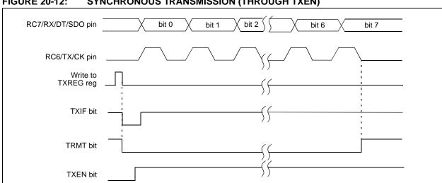
**FIGURE 20-12:** SYNCHRONOUS TRANSMISSION (THROUGH TXEN)
