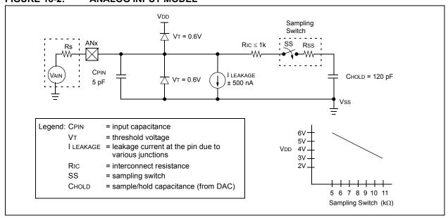
To calculate the minimum acquisition time, Equation 18-1 may be used. This equation assumes that 1/2 LSb error is used (1024 steps for the A/D). The 1/2 LSb error is the maximum error allowed for the A/D to meet its specified resolution.
