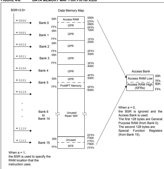
FIGURE 4-6: DATA MEMORY MAP FOR PIC18FX539
