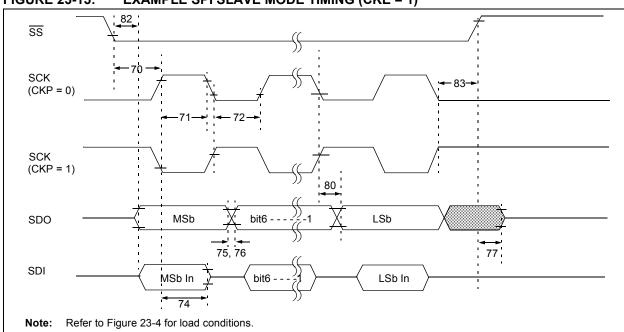
FIGURE 23-15: EXAMPLE SPI SLAVE MODE TIMING (CKE = 1)
