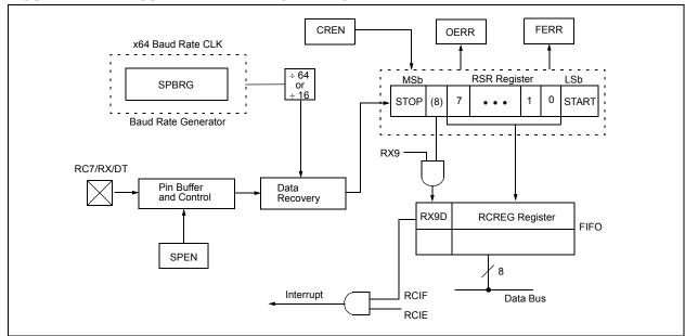
FIGURE 17-5: ASYNCHRONOUS RECEPTION
