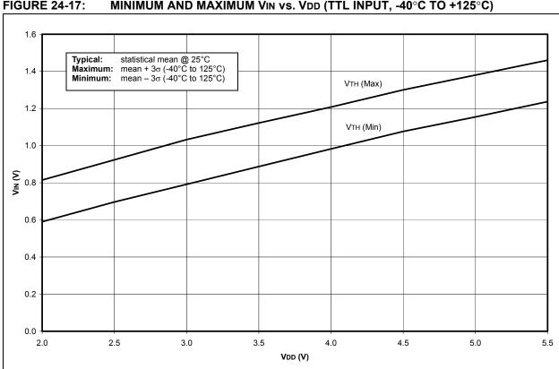
**FIGURE 24-17:** MINIMUM AND MAXIMUM VIN vs. VDD (TTL INPUT, -40°C TO +125°C)
