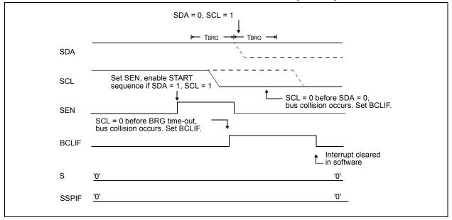
FIGURE 16-28: BRG RESET DUE TO SDA ARBITRATION DURING START CONDITION
