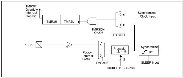
FIGURE 13-2: TIMER3 BLOCK DIAGRAM CONFIGURED IN 16-BIT READ/WRITE MODE
