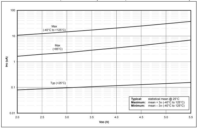
FIGURE 24-8:  $\triangle$ IBOR vs. VDD OVER TEMPERATURE (BOR ENABLED, VBOR = 2.00 - 2.16V)
