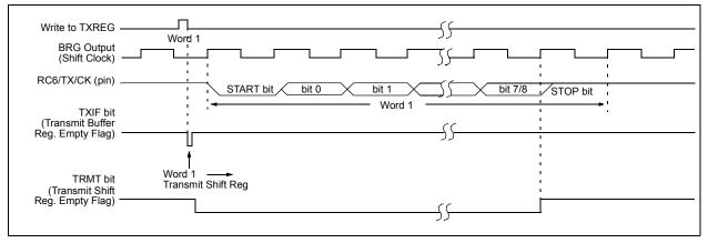
FIGURE 17-3: ASYNCHRONOUS TRANSMISSION (BACK TO BACK)
