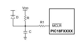
Note 1: External Power-on Reset circuit is required only if the VDD power-up slope is too slow.
