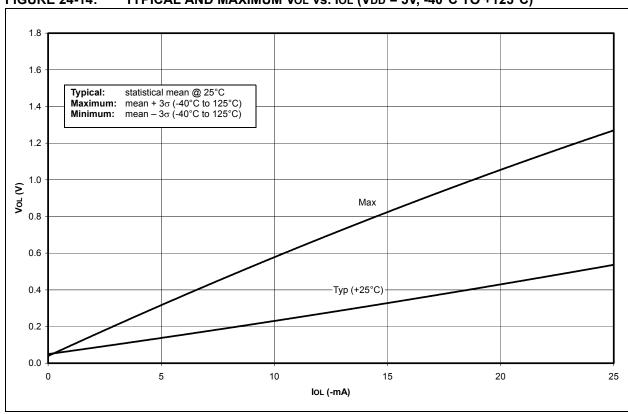
FIGURE 24-15: TYPICAL AND MAXIMUM Vol vs. Iol (VDD = 3V, -40°C TO +125°C)
