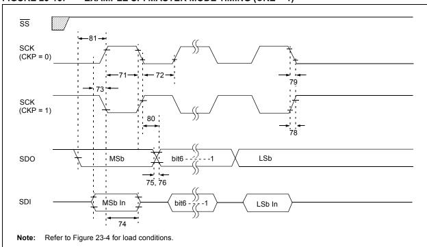
FIGURE 23-13: EXAMPLE SPI MASTER MODE TIMING (CKE = 1)
