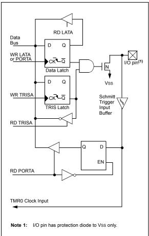
FIGURE 9-3: BLOCK DIAGRAM OF RA6 PIN
