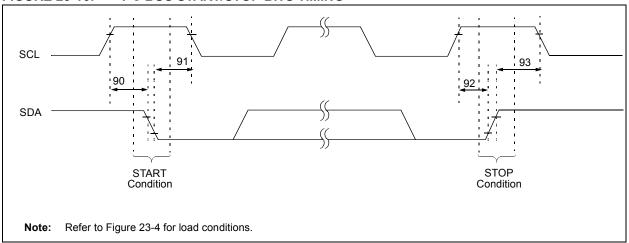
TABLE 23-15: I<sup>2</sup>C BUS START/STOP BITS REQUIREMENTS (SLAVE MODE)
