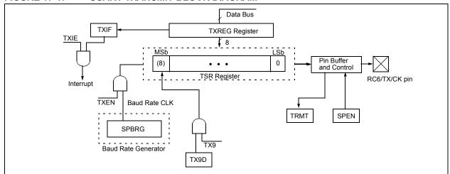
FIGURE 17-2: ASYNCHRONOUS TRANSMISSION
