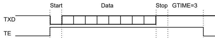
The Transmit Complete interrupt flag (INTFLAG.TXC) will be raised after the guard time is complete and TE goes low.
