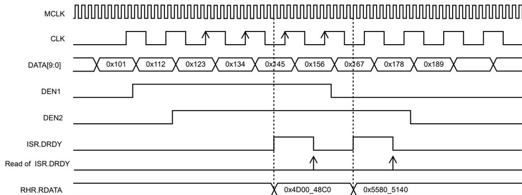
**Figure 39-6.** PCC Waveforms (DSIZE = 4\_DATA, ALWAYS = 1, HALFS = 0)
