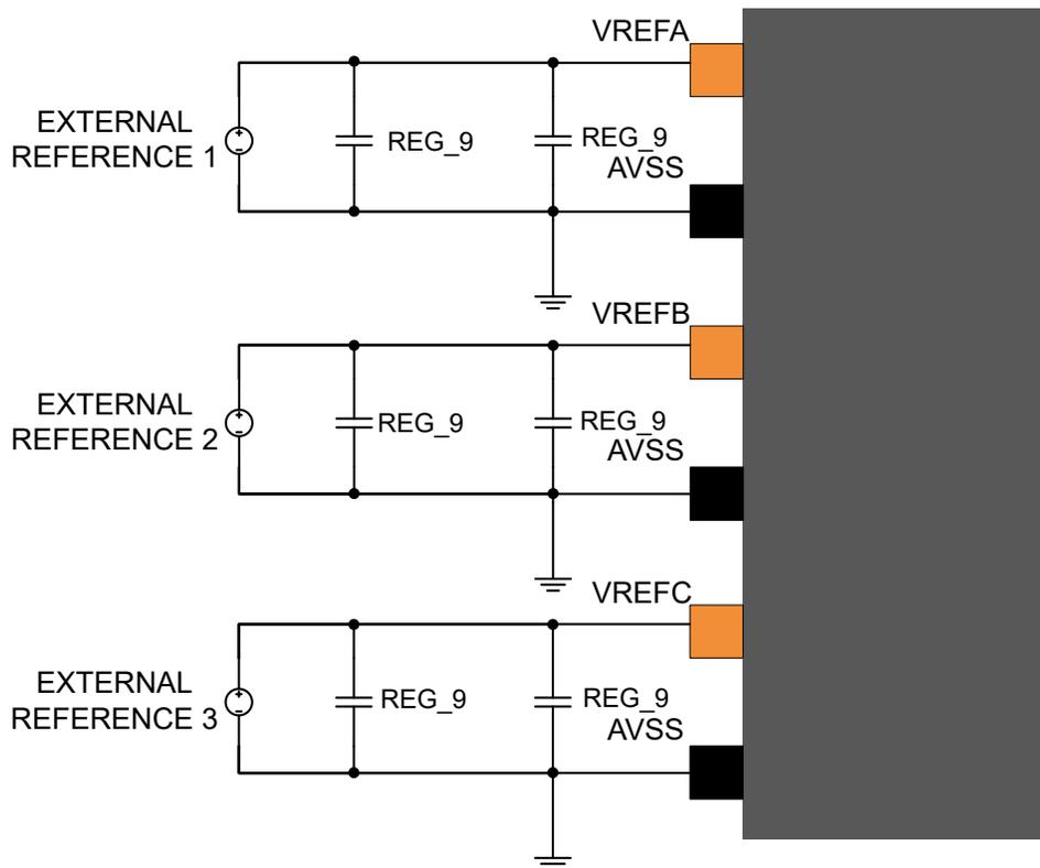
Figure 58-5. External Analog Reference Schematic With Two References
