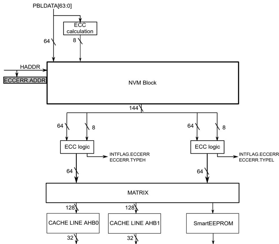
**Note:** The ECC correction is disabled when access is performed by the SmartEEPROM interface.
