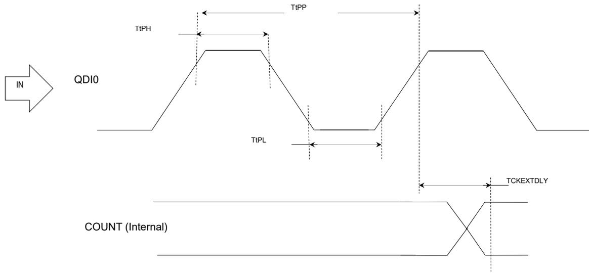
Figure 55-27. Position Decoder (PDEC) Input Timing Diagrams
