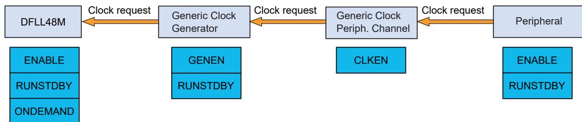
All clock sources in the system can be run in an on-demand mode: the clock source is in a stopped state unless a peripheral is requesting the clock source. Clock requests propagate from the peripheral, via the GCLK, to the clock source. If one or more peripheral is using a clock source, the clock source will be started/kept running. As soon as the clock source is no longer needed and no peripheral has an active request, the clock source will be stopped until requested again.
