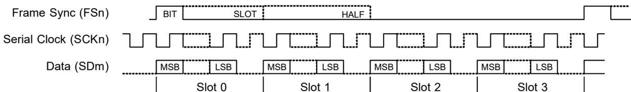
Data bits are sent on the falling edge of the Serial Clock and sampled on the rising edge of the Serial Clock. The FSn pin provides a frame synchronization signal, at the beginning of slot 0. The delay between the frame start and the first data bit is defined by writing the CLKCTRLn.BITDELAY field.
