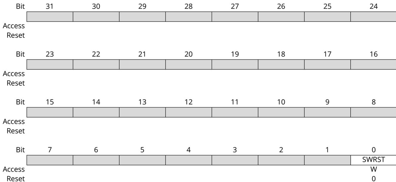
**Bit 0 – SWRST** Cache Controller Software Reset
