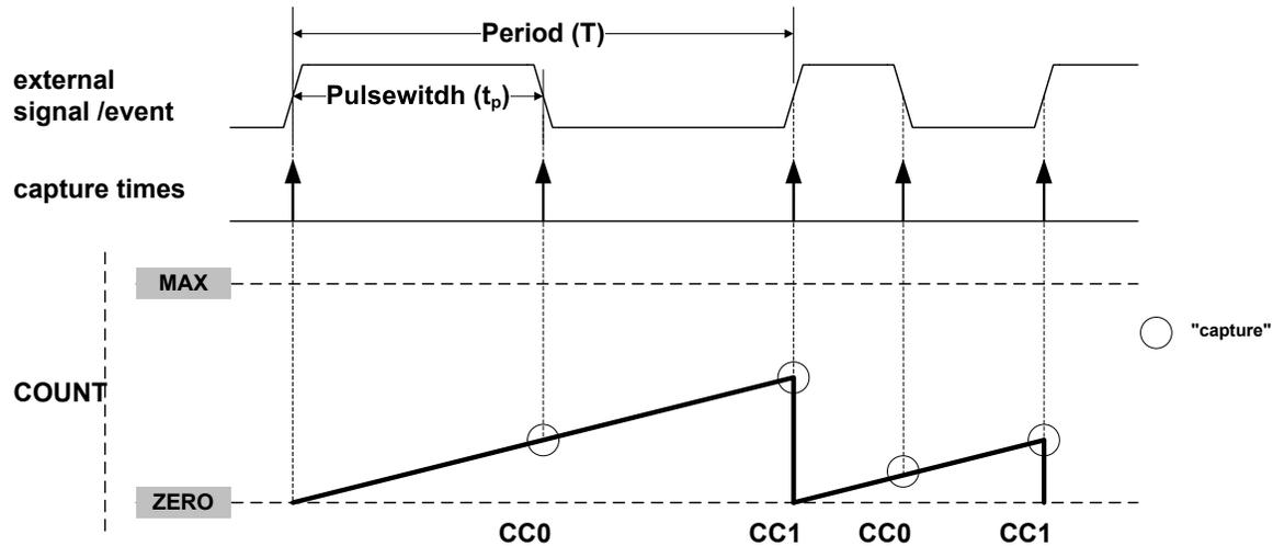
Selecting PWP or PPW in the Timer/Counter Event Input 1 Action bit group in the Event Control register (EVCTRL.EVACT1) enables the TCC to perform one capture action on the rising edge and the other one on the falling edge. When using PPW event action, period  $T$  will be captured into CC0 and the pulse-width  $t_p$  into CC1. The PWP (Pulse-width and Period) event action offers the same functionality, but  $T$  will be captured into CC1 and  $t_p$  into CC0.
