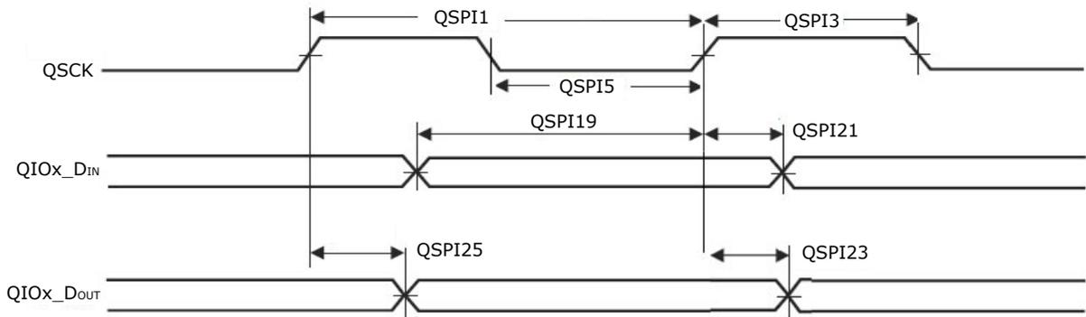
Figure 55-13. QSPI DDR Mode 0 Write Timing Diagram
