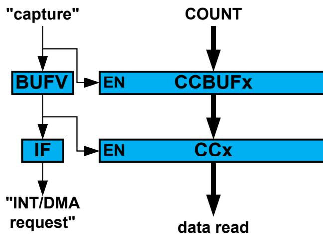
The TCC can detect capture overflow of the input capture channels. When a new capture event is detected while the Capture Buffer Valid flag (STATUS.CCBUFV) is still set, the new timestamp will not be stored and INTFLAG.ERR will be set.
