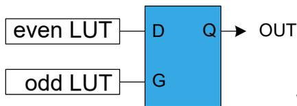
When the even LUT is disabled (LUTCTRL0.ENABLE=0 / LUTCTRL2.ENABLE=0), the latch output will be cleared. The G-input is forced enabled for one more APB clock cycle, and the D-input to zero. In all other cases, the latch output (OUT) is refreshed as shown in the following table.
