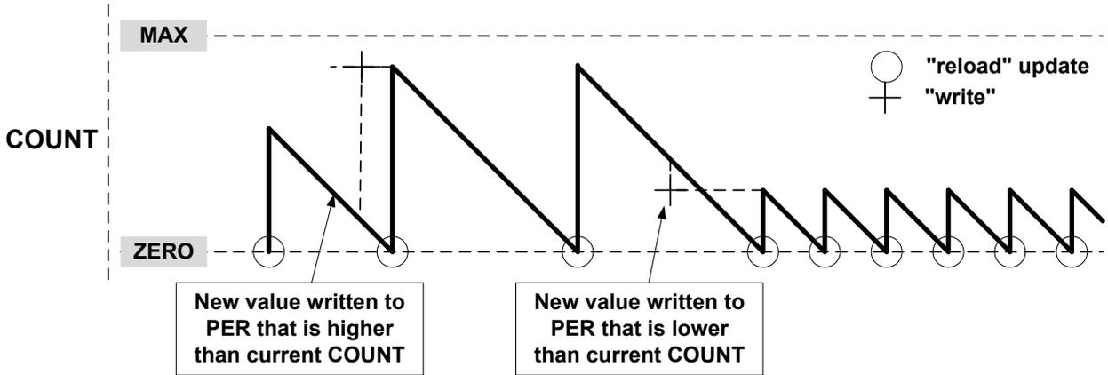
A counter wraparound can occur in any operation mode when up-counting without buffering, see the figure, above. COUNT and TOP are continuously compared, so when a new value that is lower than the current COUNT is written to TOP, COUNT will wrap before a compare match.
