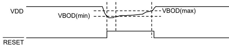
Enabling the BOD33 hysteresis by writing the Hysteresis bit field in the BOD33 register (BOD33.HYST) to a non-null value will add hysteresis to the BOD33 threshold level.
