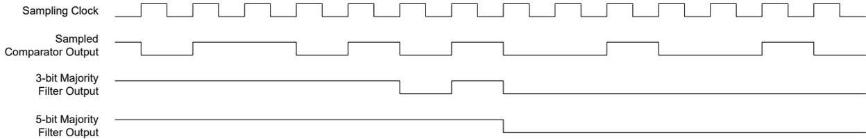
For Single-shot mode, the comparison completes after the Nth filter sample, as shown in the following figure.
