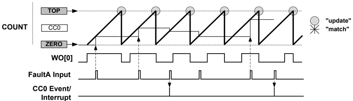
**Hardware Halt Action** This is configured by writing 0x1 to the Fault n Halt mode bits in the Recoverable Fault n Configuration register (FCTRLn.HALT). When enabled, the timer/counter is halted and the cycle is extended as long as the corresponding fault is present.
