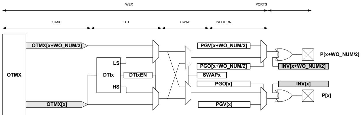
The **output matrix (OTMX)** unit distributes compare channels, according to the selectable configurations in the following table.
