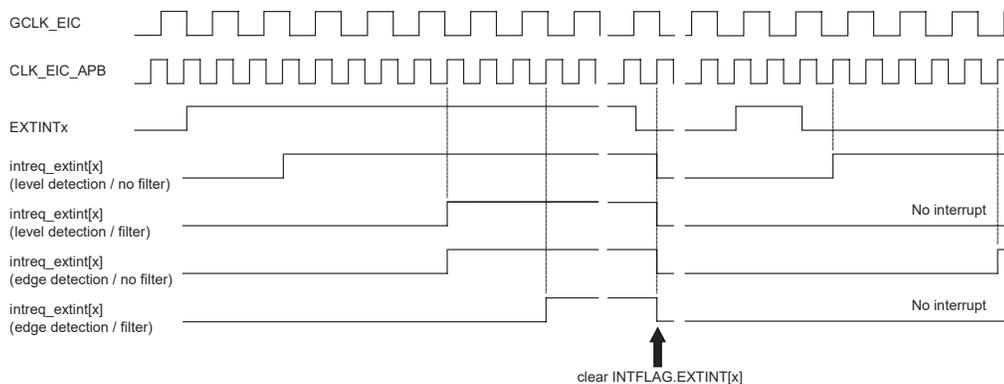
Detection latency depends on the detection mode.
