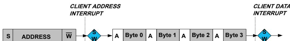
The LENGTH register can be written before the frame begins, or when the AMATCH interrupt is set. If the frame size is not LENGTH.LEN Bytes, the Length Error status bit (STATUS.LENERR) is raised. If
