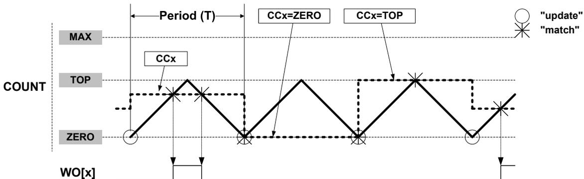
Using dual-slope PWM results in a lower maximum operation frequency compared to single-slope PWM generation. The period (TOP) defines the PWM resolution. The minimum resolution is 1 bit (TOP=0x00000001).
