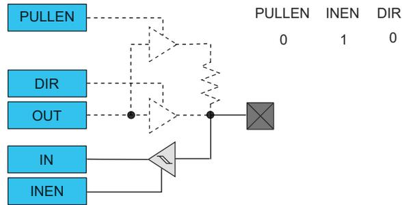
Figure 29-5. I/O Configuration - Input with Pull
