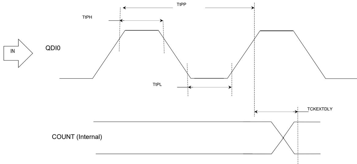
Figure 56-18. Position Decoder (PDEC) Input Timing Diagrams
