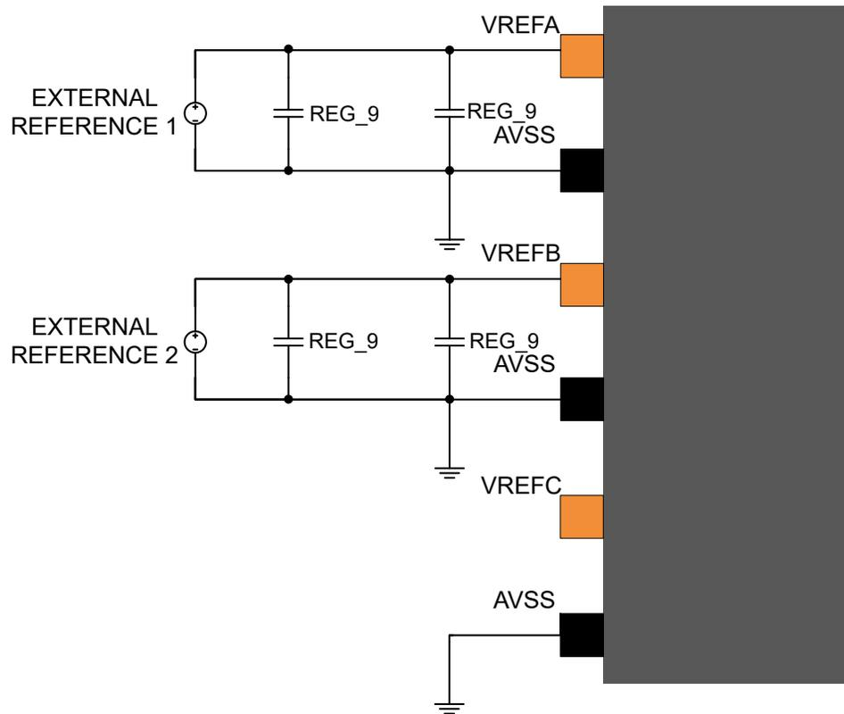
Figure 58-6. External Analog Reference Schematic With One Reference
