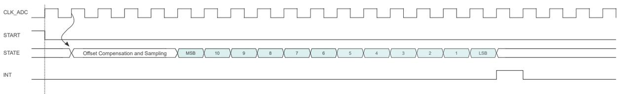
The following figure shows the ADC timing for free-running mode conversion.
