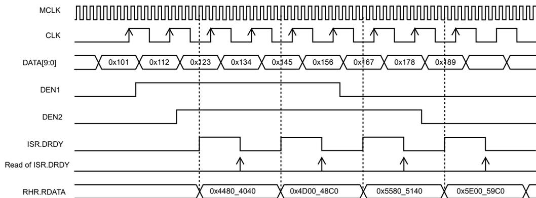
**Figure 39-9.** PCC Waveforms (DSIZE = 4\_DATA, ALWAYS = 0, HALFS = 1, FRSTS = 0)
