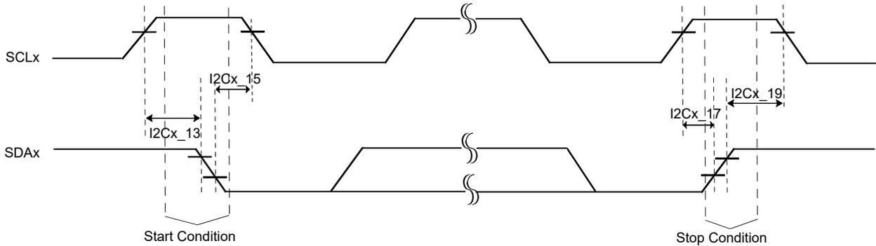
Figure 55-11. I<sup>2</sup>C Bus Data Client Mode Timing Diagrams
