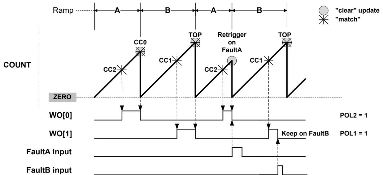
Figure 45-21. RAMP2 Critical Operation With 2 Channels
