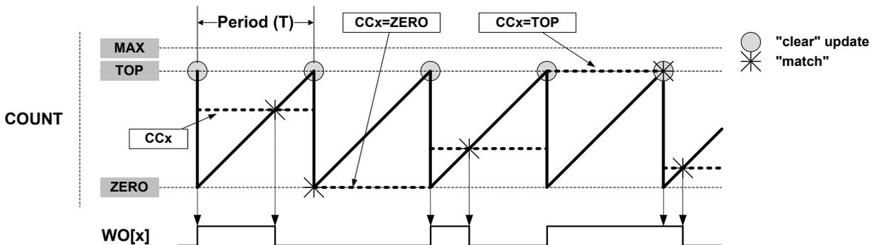
The following equation calculates the exact resolution for a single-slope PWM ( $R_{P_{PWM\_SS}}$ ) waveform:
