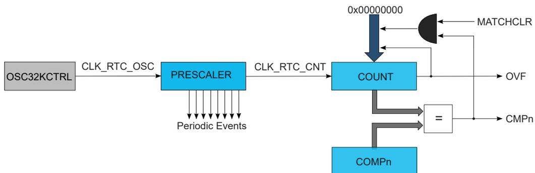
Figure 23-2. RTC Block Diagram (Mode 1 — 16-Bit Counter)
