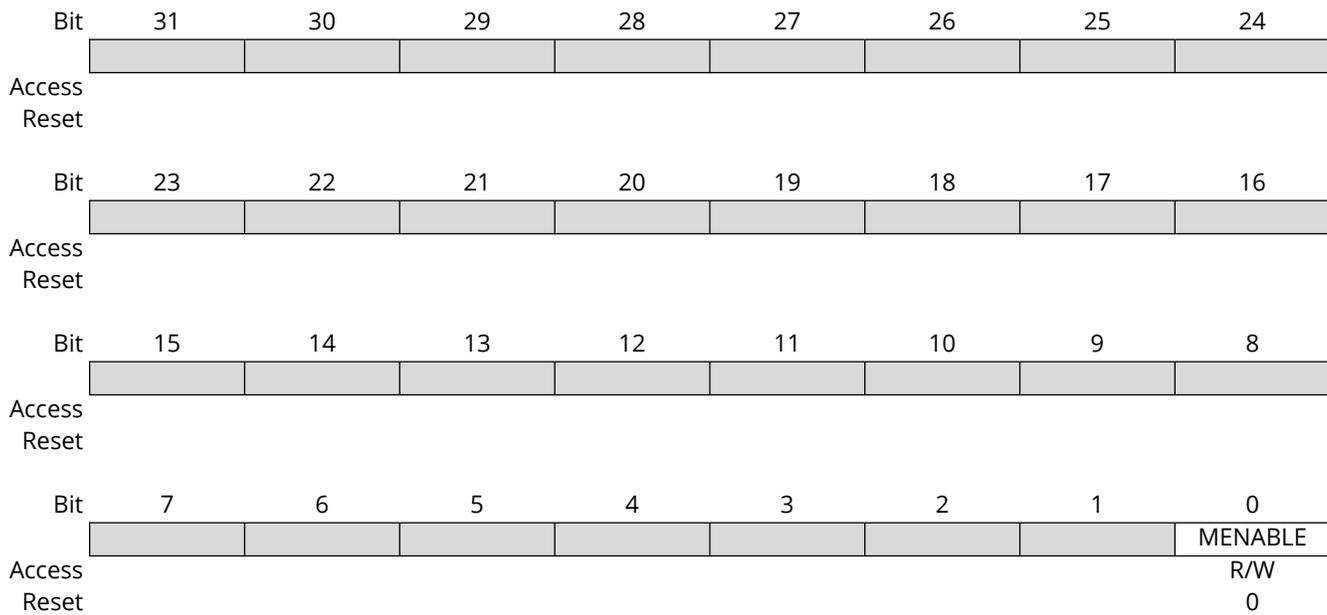
**Bit 0 – MENABLE** Cache Controller Monitor Enable
