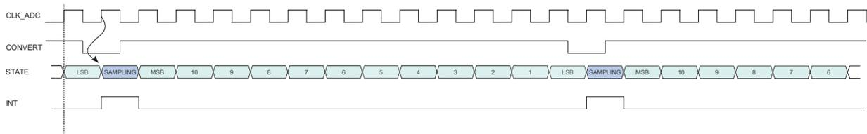
In free running mode, the sampling rate  $R_S$  is calculated by:
