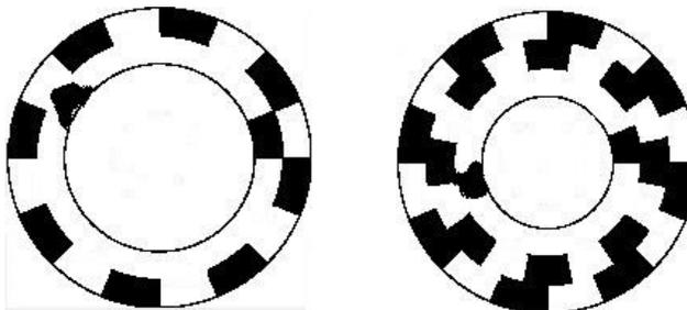
**Type 3 Error: Missing Angular Step Detection**
