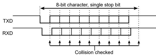
The figure below shows the conditions for a collision detection. In this case, the Start bit and the first Data bit are received with the same value as transmitted. The second received Data bit is found to be different than the transmitted bit at the detection point, which indicates a collision.
