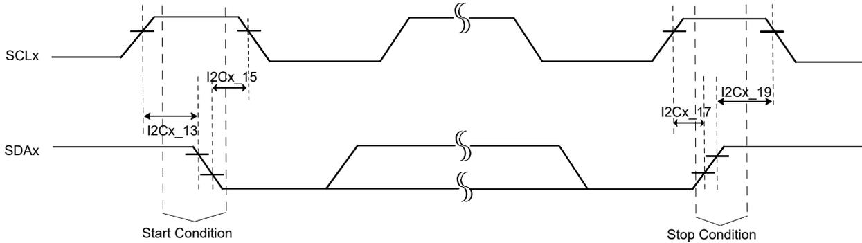
Figure 55-9. I<sup>2</sup>C Bus Data Host Mode Timing Diagrams
