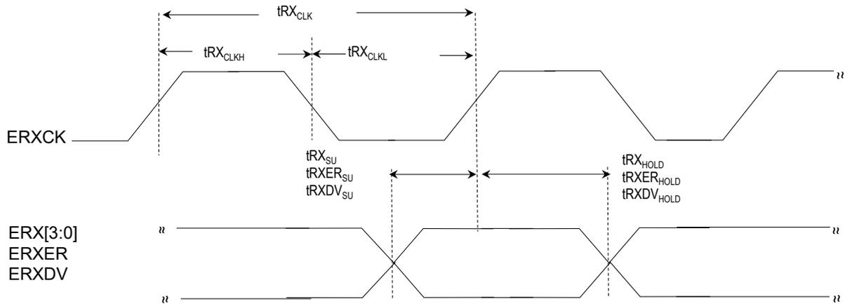
Figure 55-24. MII Transmit Ethernet Module Timing Diagram (Media-Independent Interface)
