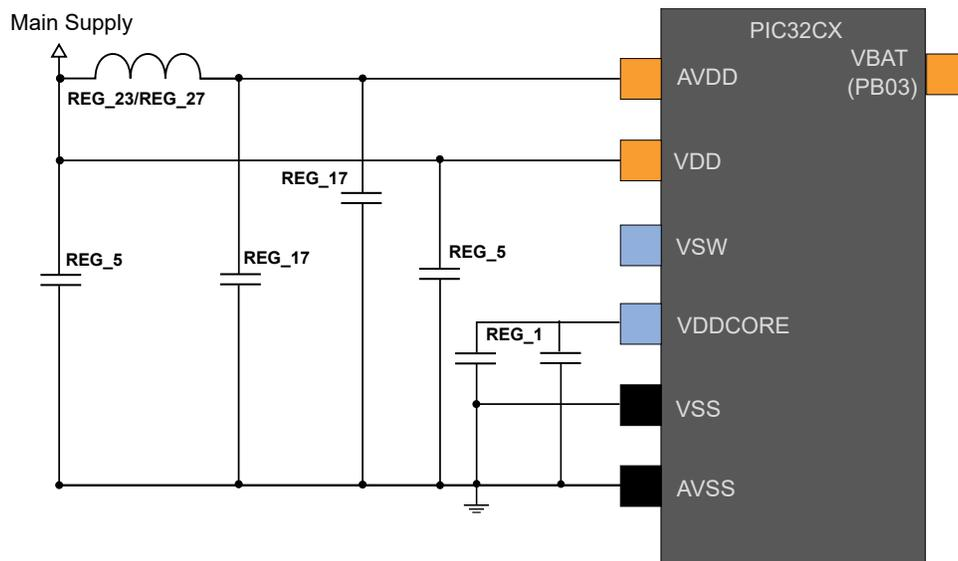
Figure 58-3. Power Supply Connection for Battery Backup Mode
