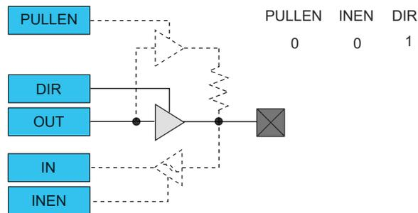
Figure 29-7. I/O Configuration - Totem-Pole Output with Enabled Input
