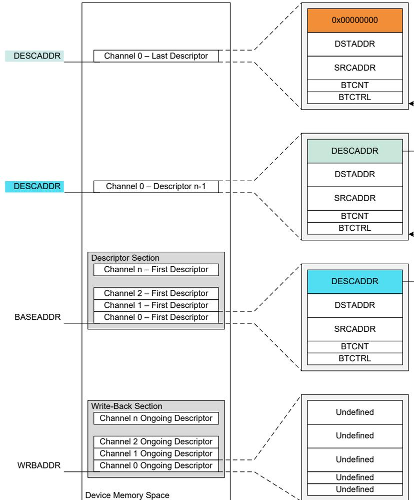
The size of the descriptor and write-back memory sections are dependent on the number of the most significant enabled DMA channel  $m$ , as shown below:
