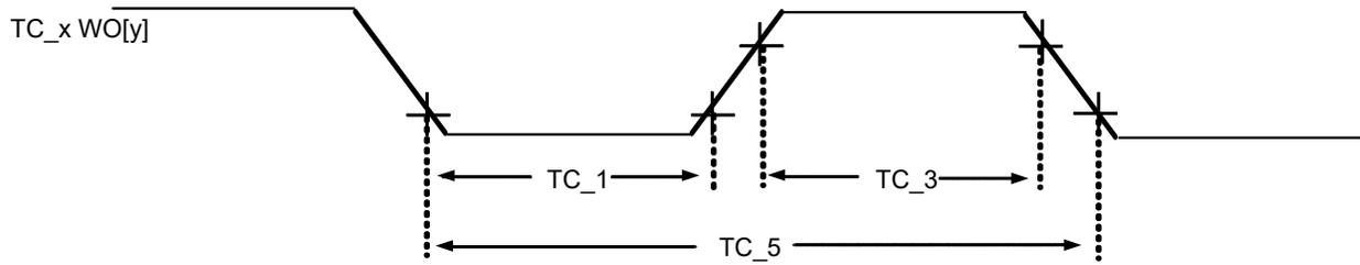
Figure 56-12. TC Timer Compare Output Module Timing Diagrams
