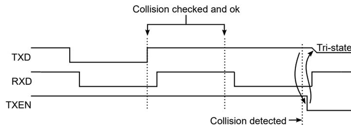
When a collision is detected, the USART follows these steps:
