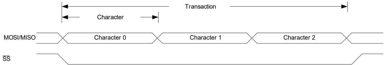
The SPI Host must pull the SPI select line ( $\overline{SS}$ ) of the desired Client low to initiate a transaction if multiple Clients are connected to the bus. The SPI select line can be wired low if there is only one SPI Client on the bus. The Host and Client prepare data to send through their respective Shift registers, and the Host generates the serial clock on the SCK line.
