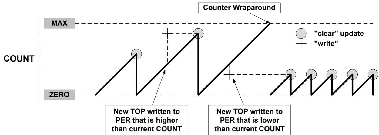
A counter wraparound can occur in any operation mode when up-counting without buffering, see the following figure.
