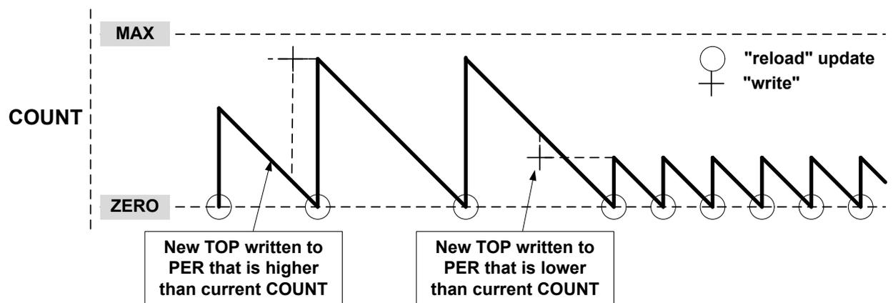
When double buffering is used, the buffer can be written at any time and the counter will still maintain correct operation. The period register is always updated on the update condition, as shown in the following figure. This prevents wraparound and the generation of odd waveforms.
