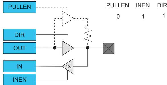
Figure 29-8. I/O Configuration - Output with Pull
