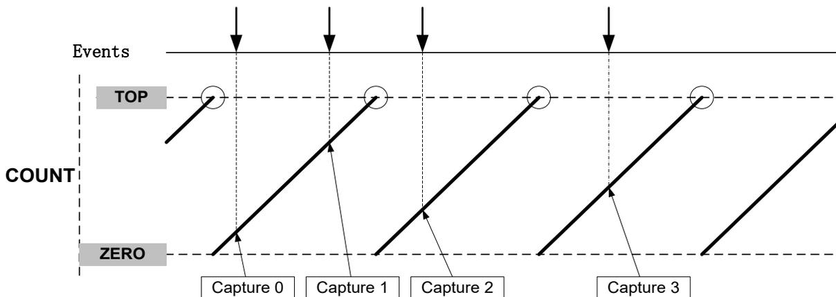
The TC can detect capture overflow of the input capture channels: When a new capture event is detected while the Capture Interrupt flag (INTFLAG.MCx) is still set, the new timestamp will not be stored and INTFLAG.ERR will be set.
