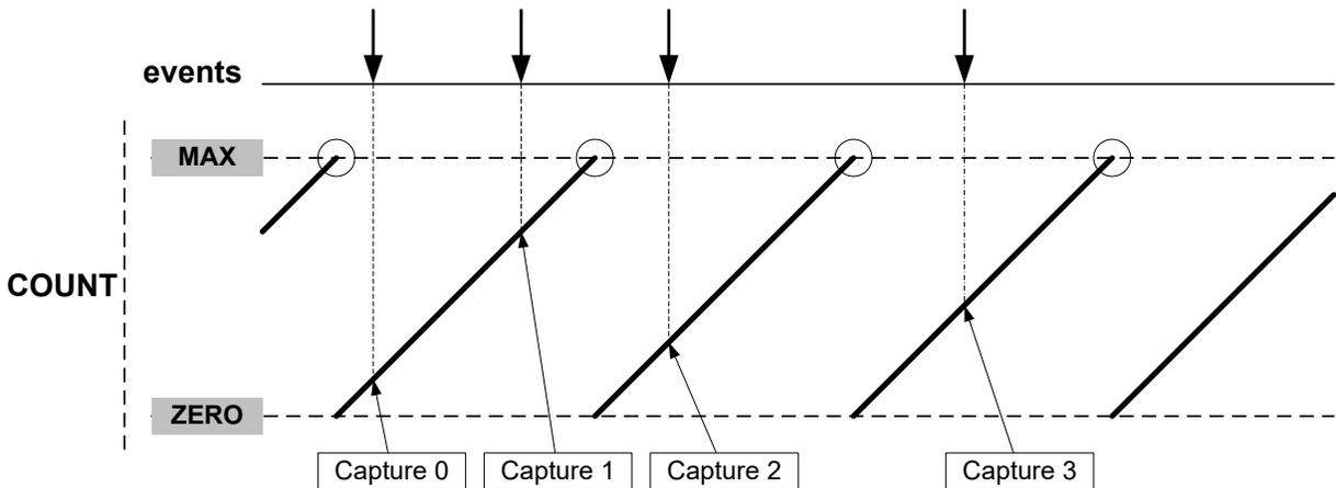
For input capture, the Buffer register and the corresponding CCx act like a FIFO. When CCx is empty or read, any content in CCBUFx is transferred to CCx. The Buffer Valid flag is passed to set the CCx Interrupt flag (IF) and generate the optional interrupt, event, or DMA request. The CCBUFx register value cannot be read, all captured data must be read from the CCx register.
