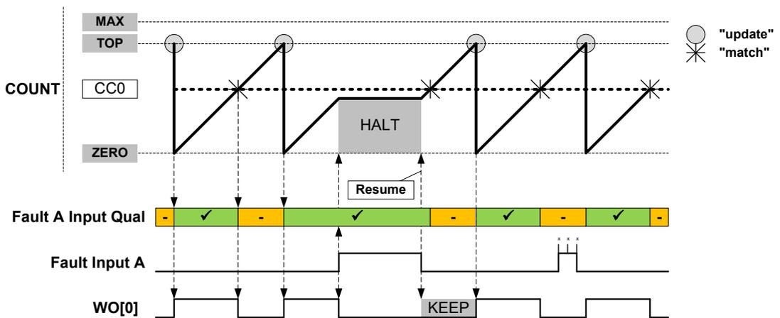
**Software Halt Action** This is configured by writing 0x2 to the Fault n Halt mode bits in the Recoverable Fault n configuration register (FCTRLn.HALT). Software halt action is similar to hardware halt action, but in order to restart the timer/counter, the corresponding fault condition must not be present anymore, and the corresponding FAULT n bit in the STATUS register must be cleared by software.
