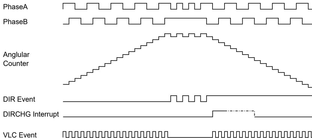
To avoid spurious interrupts when coding wheel is stopped, the direction change condition is reported as an interrupt, only on the second edge confirming the direction change.
