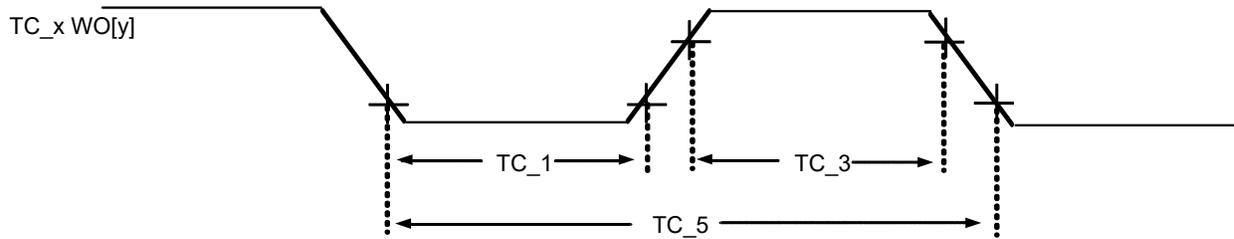
Figure 55-17. TC Timer Compare Output Module Timing Diagrams
