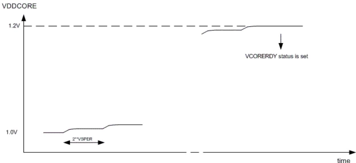
The STATUS.VCORERDY bit is set to '1' as soon as the VDDCORE voltage has reached the target voltage. During voltage transition, STATUS.VCORERDY will read '0'. The Voltage Ready interrupt (VCORERDY) can be used to detect a 0-to-1 transition of STATUS.VCORERDY, see also "Interrupts".
