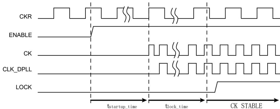
**Figure 18-6.** CK and CLK\_DPLL Output from Running Mode to DPLL Off Mode.
