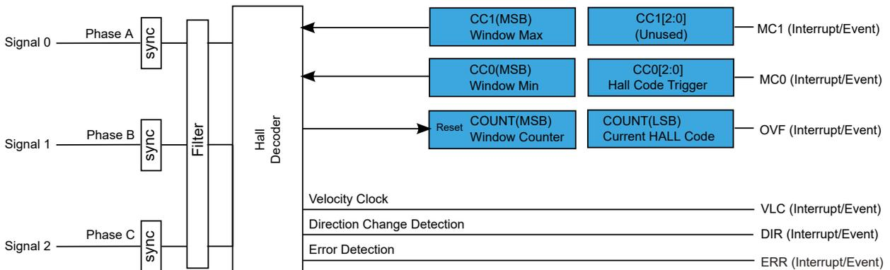
When positive rotation is detected, the DIR status bit is set (STATUS.DIR = 1). When a negative rotation sequence is detected, the DIR status bit is set (STATUS.DIR = 0).
