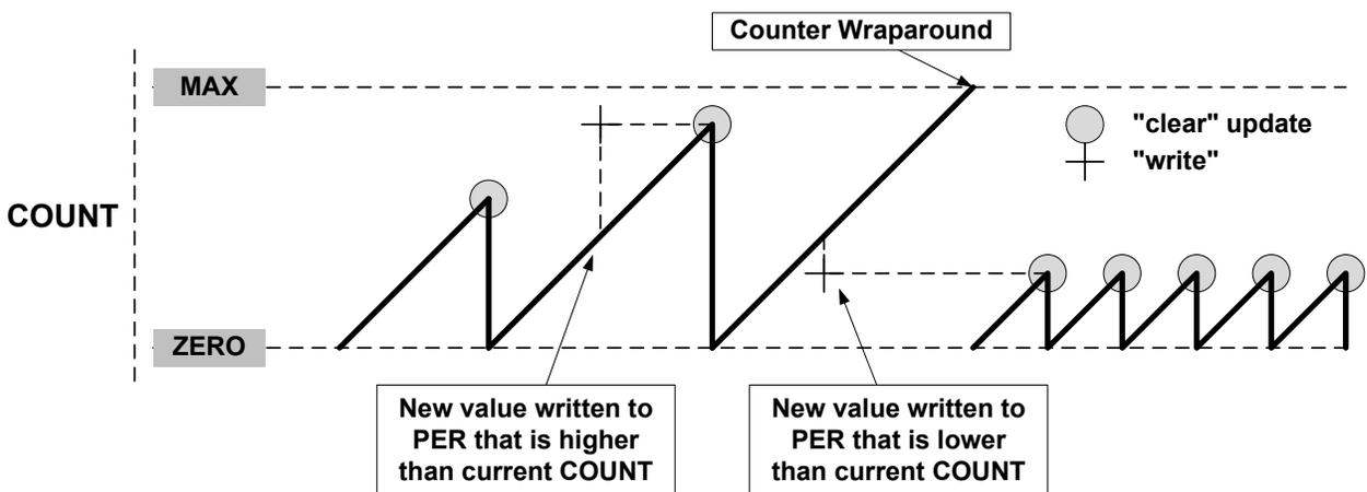
Figure 45-11. Unbuffered Single-Slope Down-Counting Operation
