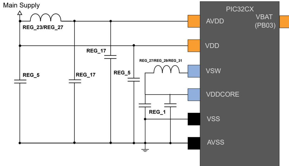
Figure 58-2. Power Supply Connection for Linear Mode Only
