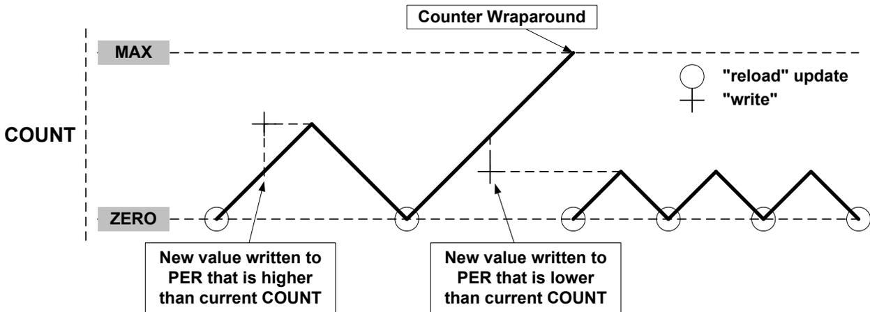
When double buffering is used, the buffer can be written at any time and the counter will still maintain correct operation. The period register is always updated on the update condition, as shown in the following figure. This prevents wraparound and the generation of odd waveforms.
