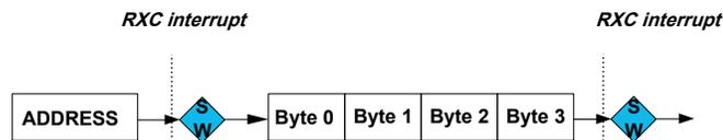
When utilizing the length counter, the LENGTH register must be written before the frame begins. If the frame length while SS is low is not a multiple of LENGTH.LEN Bytes, the Length Error Status bit (STATUS.LENERR) is raised. If LENGTH.LEN is not a multiple of 4 Bytes, the final INTFLAG.RXC interrupt will be raised when the last Byte is received.
