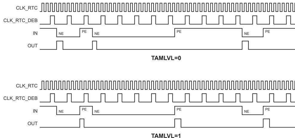
**Figure 23-6. Edge Detection with Synchronous Stability Debouncing**
