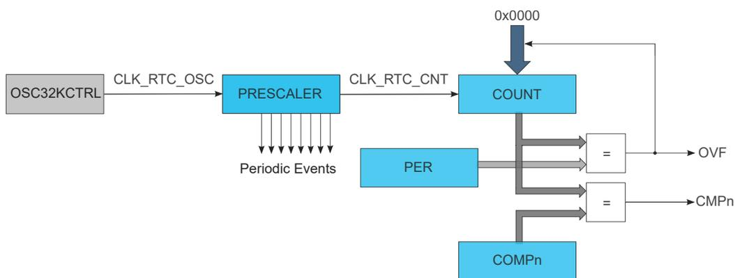
Figure 23-3. RTC Block Diagram (Mode 2 — Clock/Calendar)
