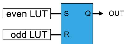
When the even LUT is disabled LUTCTRL0.ENABLE=0 / LUTCTRL2.ENABLE=0), the latch output will be cleared. The R-input is forced enabled for one more APB clock cycle and S-input to zero. In all other cases, the latch output (OUT) is refreshed as shown in the following table.
