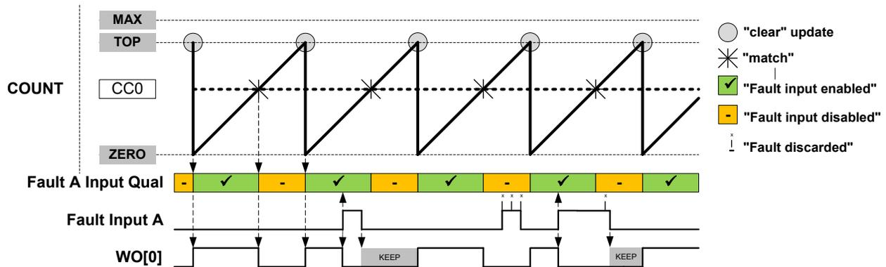
**Restart Action** This is enabled by writing the Fault n Restart bit in Recoverable Fault n Configuration register (FCTRLn.RESTART) to '1'. When enabled, the timer/counter will be restarted as soon as the corresponding fault condition is present. The ongoing cycle is stopped and the timer/counter starts a new cycle, see the following figure. In Ramp 1 mode, when the new cycle starts, the compare outputs will be clamped to inactive level as long as the fault condition is present.
