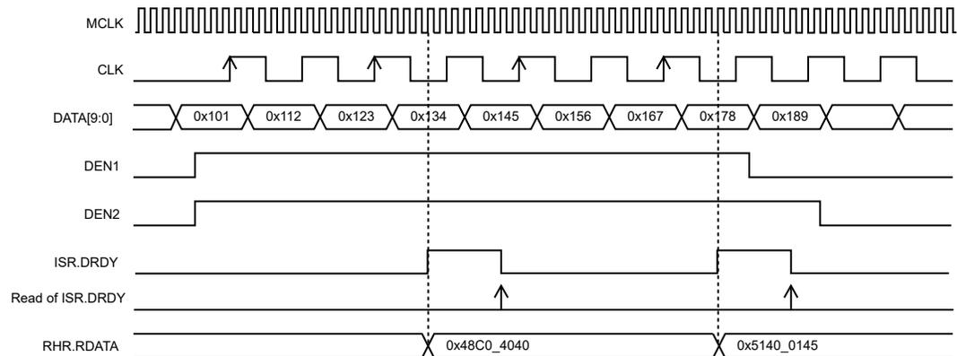
**Figure 39-12.** PCC Waveforms (DSIZE = 4\_DATA, ALWAYS = 0, HALFS = 1, FRSTS = 1)
