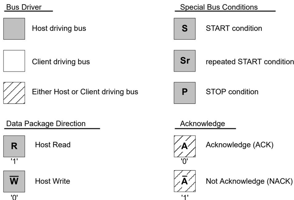
Figure 34-3. Basic I<sup>2</sup>C Transaction Diagram
