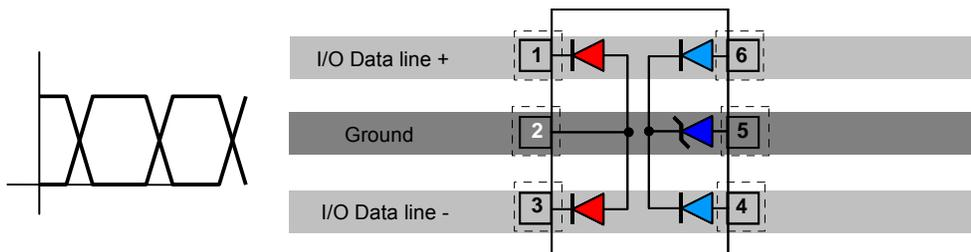
Line-line concept ease the PCB design, directly placing the device over the data lines, opening only the contact points. VREF is fixed by the operating voltage, referenced to the ground.
