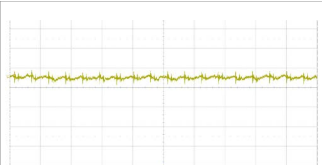
Output voltage ripple at: T_{P1} = +25^\circ\text{C} , V_I = 110\text{ V} , I_O = 6\text{ A} resistive load. Trace: output voltage (20 mV/div.). Time scale: (5 μs/div.). 20MHz bandwidth
