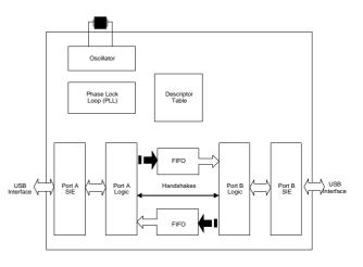
As shown in the block diagram above, this ASIC contains two USB units working independently. Together with the two FIFOs and control logic in between, they exchange data without blocking. The entire clock oscillator, PLL, voltage regulators, USB transceivers, and power-on reset circuits are integrated on the chip. There is no glue logic needed.
