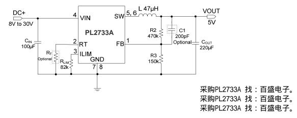
\* The output voltage is set by R2 and R3:  $V_{OUT}$  = 1.21V • [1 + (R2/R3)].
