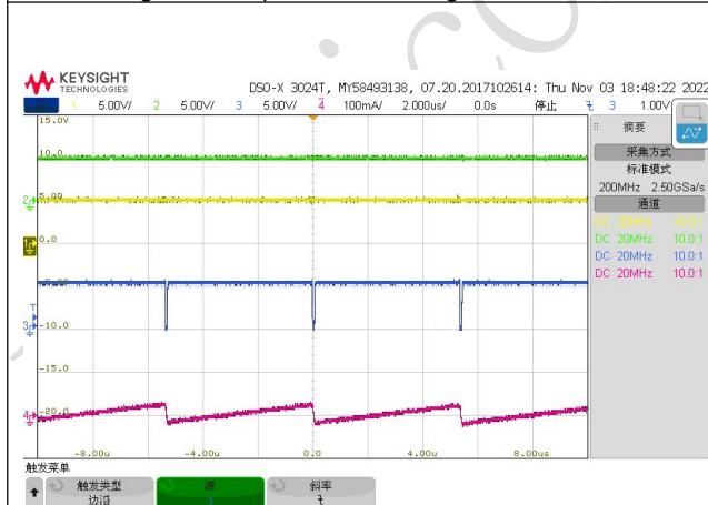
Fig.14 Start up waveform through EN, Iout =0A
