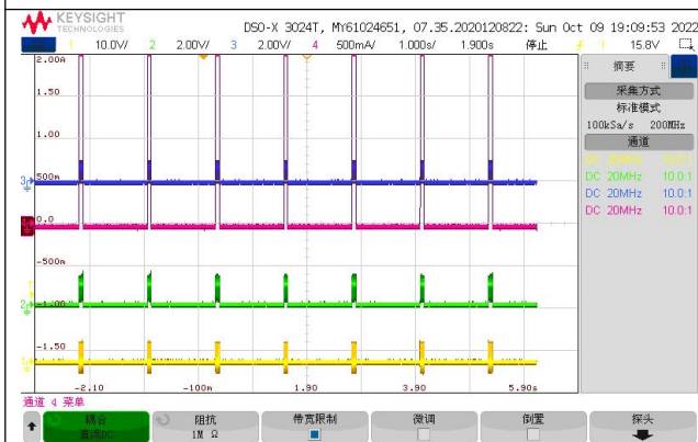
Fig.28 Load Transient IOUT=0.5-1.5A I-ramp=0.5A/us
