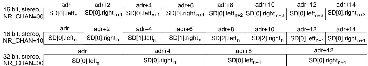
Figure 2: Examples of Audio Out Memory DMA Formats
