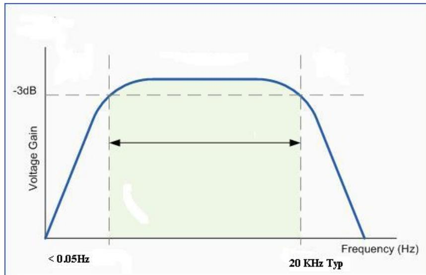
Fig. 2 Typical Bode Plot for EPIC ECG Sensor
