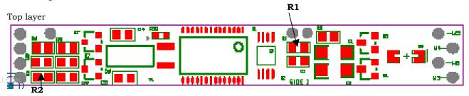
The R2 'pack thermistor' or T-pin' signal is used by external devices, such as chargers, to determine the chemistry of the battery pack or it's temperature (using and external circuit.) The P3 module includes this T-pin' value at R2 as one of two values. As shown in the parts list, this may be either a NTC thermistor (same as R1) for NiMH applications or it may be a 365 ohm resistor for Li Ion applications.
