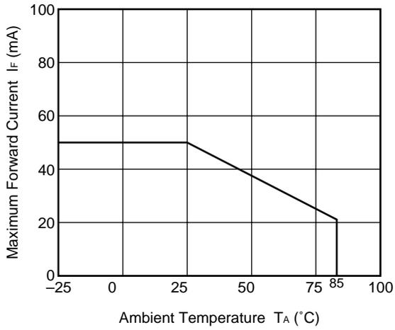
MAXIMUM LOAD CURRENT vs. AMBIENT TEMPERATURE
