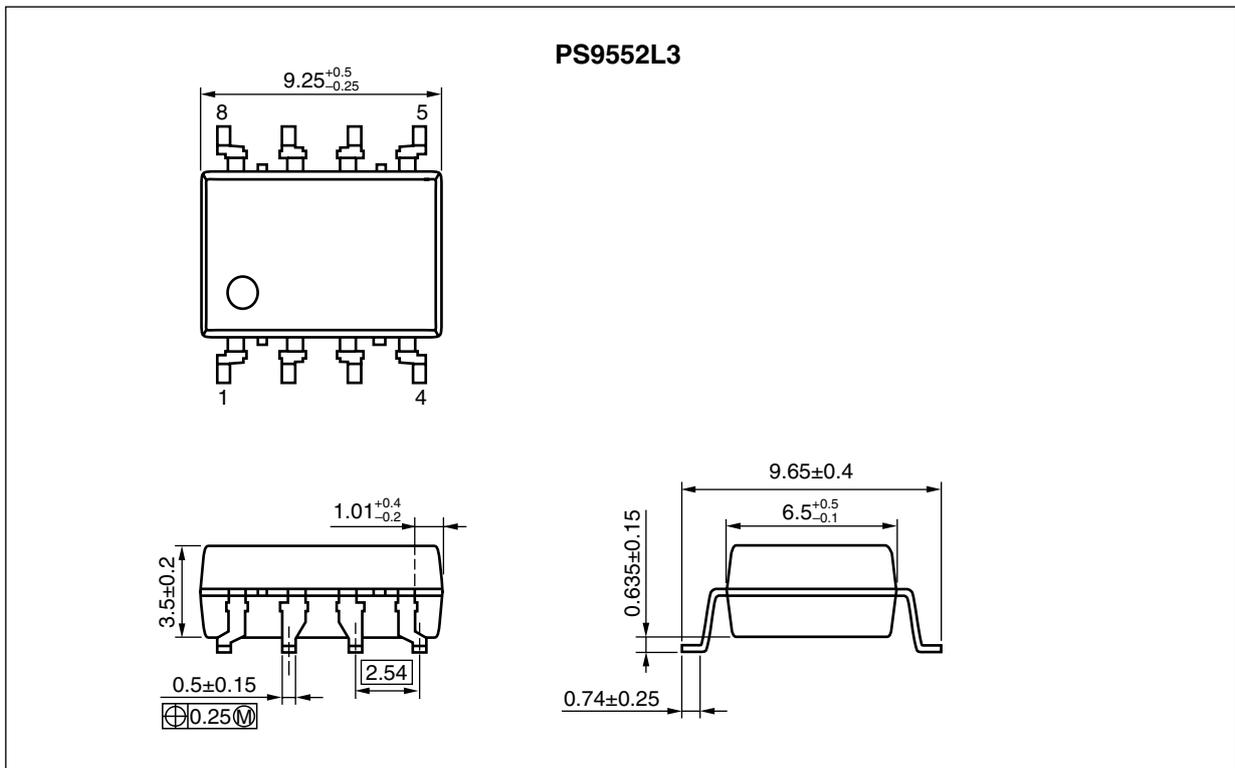
Lead Bending Type For Long Creepage Distance
