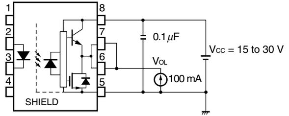
Fig. 5 I<sub>FLH</sub> Test Circuit
