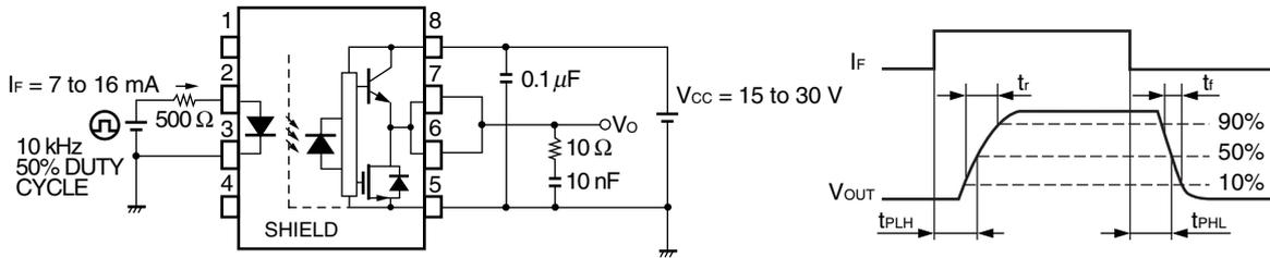
Fig. 8 CMR Test Circuit and Wave Forms
