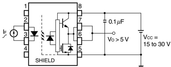
Fig. 6 UVLO Test Circuit
