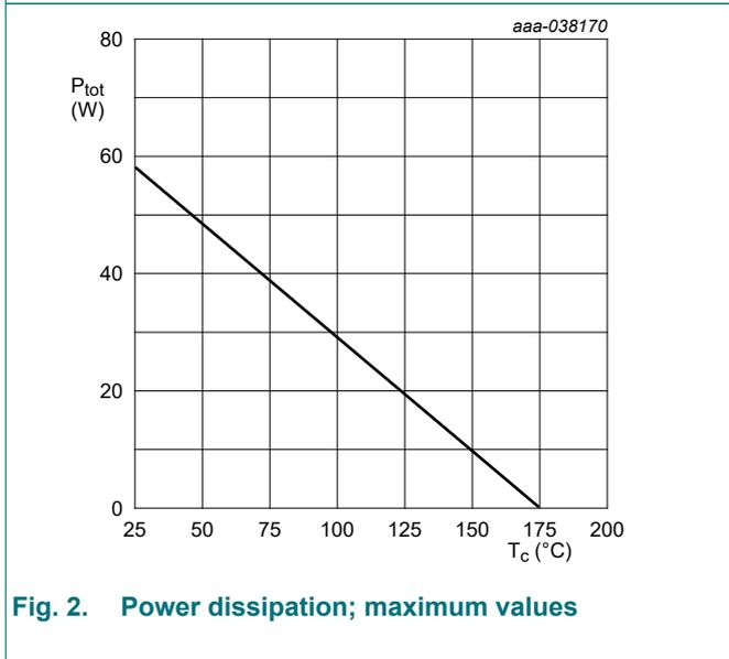
Fig. 2. Power dissipation; maximum values
