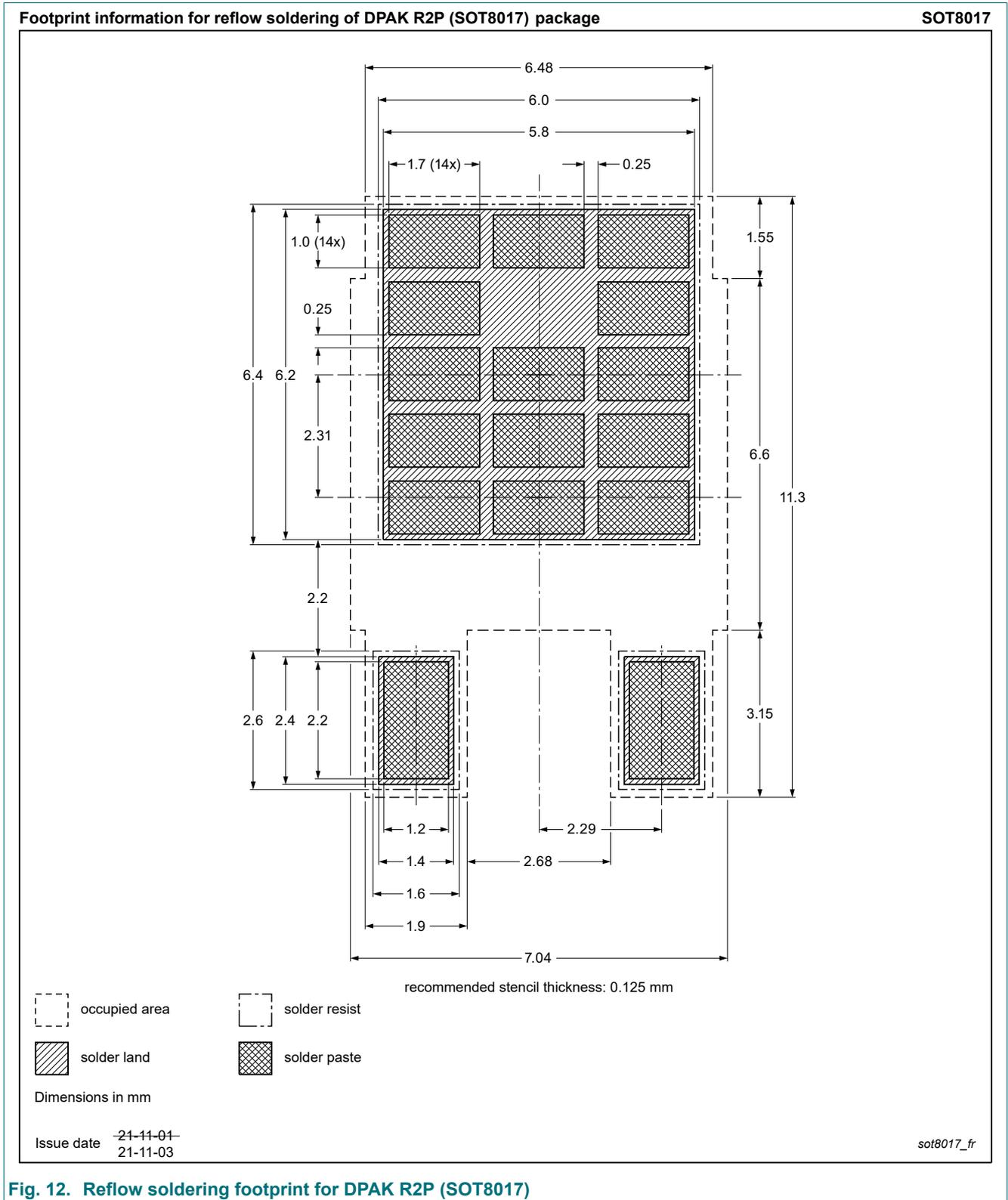
**Fig. 12. Reflow soldering footprint for DPAK R2P (SOT8017)**
