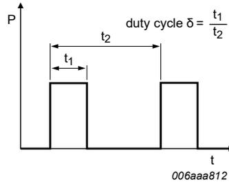
Fig. 10. Duty cycle definition
