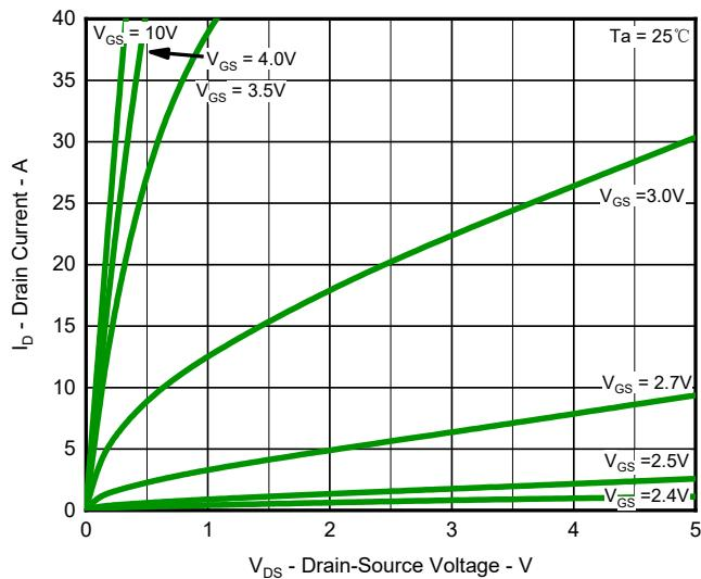
Fig.1 Output Characteristics
