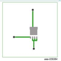
70 µm thick copper on FR4 board
