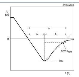
Fig. 5. Reverse recovery timing definition
