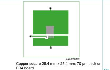
Fig. 2. PCB layout for resistance from junction to ambient
