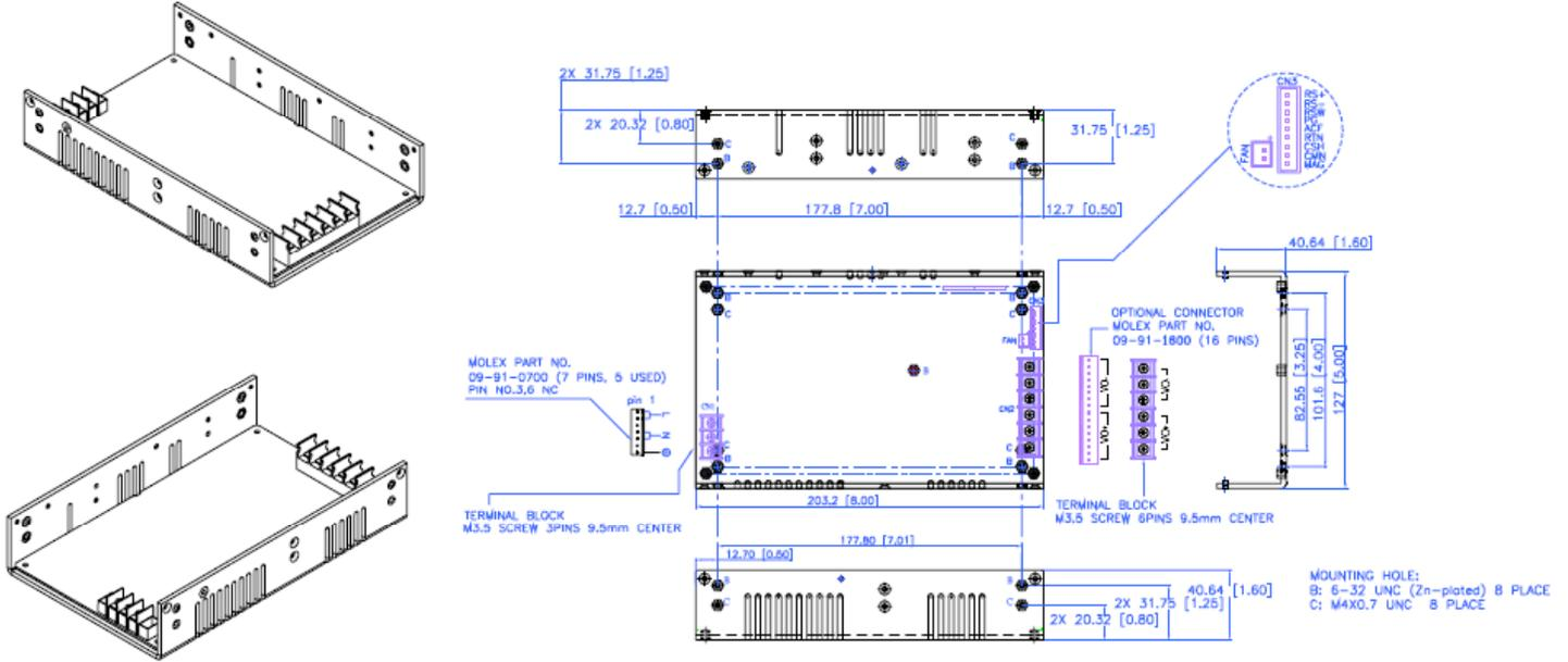
**PSRL0402E Series (Enclosed with built-in Fan Type): 9(L) x 5(W) x 1.6(H) inches; Weight: 1.6kg.**
