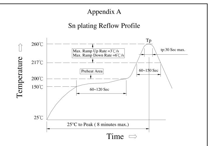
(1) Reflow Soldering Method :
