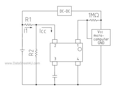
3 Battery checker (LED ON for high voltage)
