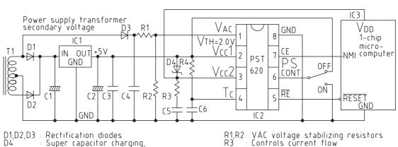
Super capacitor charging, reverse current prevention shot key barrier diode
