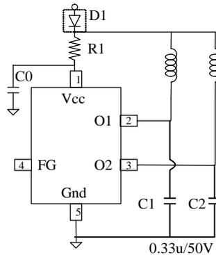
C0: decoupling capacitor 0.1uF~2.2uF (recommended)
