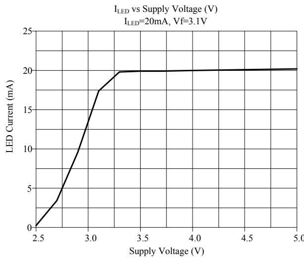
Note: Vf is the forward Voltage of LED
