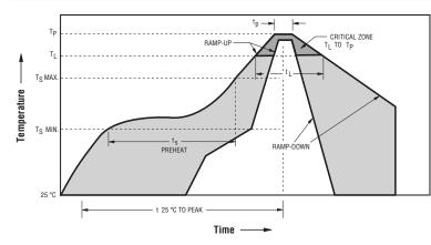
Ramp-up rate = 3 °C/sec. max. Ramp-down rate = 6 °C/sec. max.  $T_L = 217 \ ^{\circ}C$   $t_L = 60-150 \ sec.$  $T_p = 250 \text{ °C } \pm 3 \text{ °C}$ Time within 5 °C of actual Peak Temp  $(t_p)2 = 20~40$  sec.  $T_{S} min = 150 °C$  Ts max = 200 °C  $T_{S}$  min to  $T_{S}$  max = 60-180 sec., 25 °C to Peak Temperature = 8 min. max.
