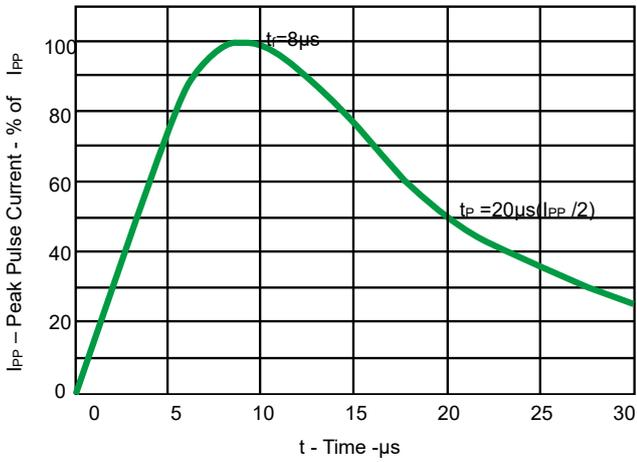
Fig 1. Pulse Waveform
