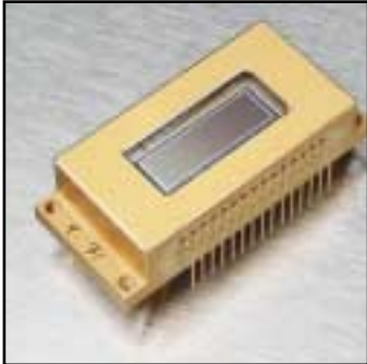
Cooled CCD Sensor— 24 μm sq. pitch, 1100x330 pixel configuration
