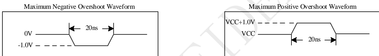
Figure 5-2 Input Test Waveforms and Measurement Level
