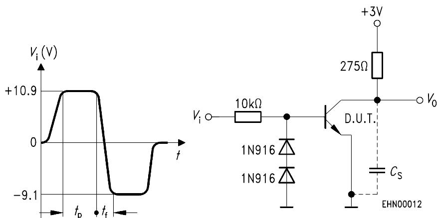
Input waveform;  $t_f < 1$  ns;  $10 \mu s < t_p \leq 500 \mu s$ ;
