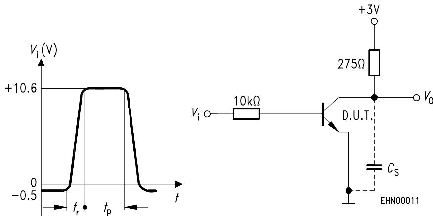
Input waveform;  $t_r < 1$  ns;  $t_p = 300$  ns;
