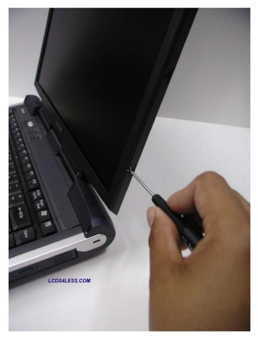
• After removing each of the screws, starting at the bottom of the display assembly insert your fingers to unsnap the front bezel. Usually it will easily snap off. If the front bezel does not easily snap off, work the plastic in different directions until it unsnaps.
