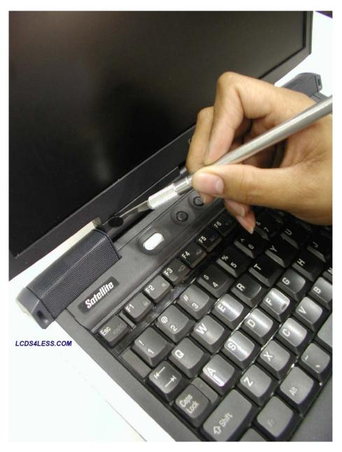
• Remove screw covers from side of display assembly if any.
