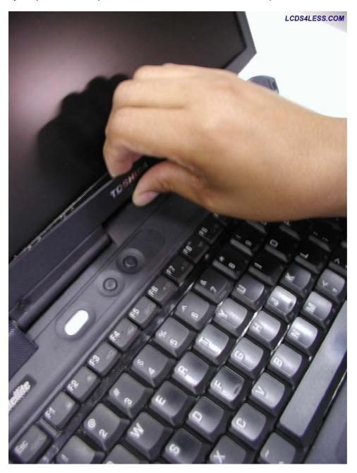
After unsnapping the front bezel from the bottom of the display assembly work your fingers around the other sides. When you have worked your fingers around the display assembly to where the latch is located, you may or may not have to slide the latch in order to detach the front bezel.
