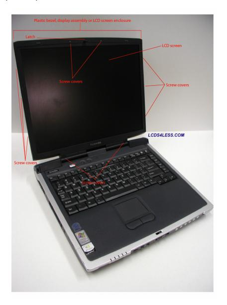
• The following Toshiba Satellite model has 2 screw covers at the bottom of the display assembly facing the user and 3 screw covers on each side of the display assembly.
