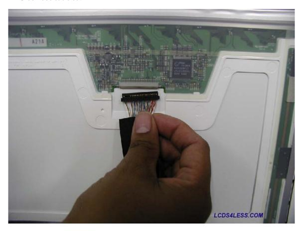
The inverter is a small device which provides the LCD screen with power. The inverter cable
