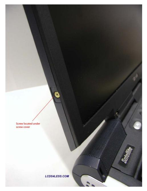
• Unscrew each of the screws securing the front plastic bezel to the display assembly.
