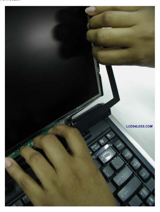
• Display assembly after front plastic bezel has been removed.
