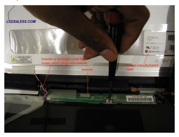
• Slide inverter cable out of inverter.
