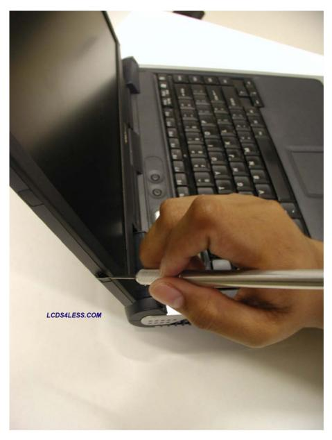
• Underneath each of the screw covers should be a small phillips screw as shown below.
