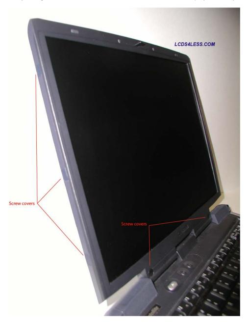
• Use a knife or some other sharp object like an exacto blade to pick off all the screw covers.
