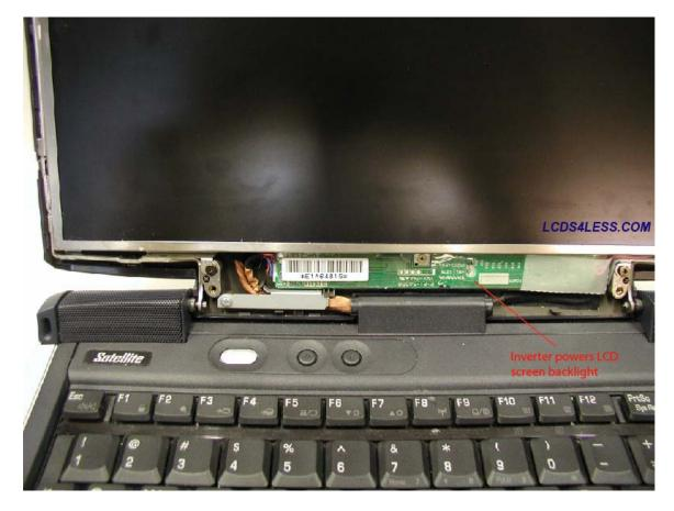
• Tilt the LCD screen forward. If you are unable to tilt the screen forward, you may have to remove the screws from an internal bracket.
