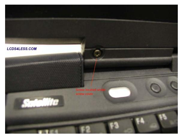
• Example of screw located under screw cover on side of display assembly.
