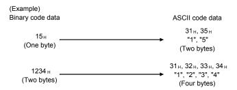
(3) The size of data that can be communicated between the Ethernet module and an external device at a time is determined by the function used and the data code (binary/ASCII) that is set by selecting [GX Developer] – [Communication data code].
