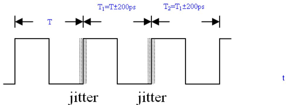
Note (2) The SSCG (Spread spectrum clock generator) is defined as below figures.
