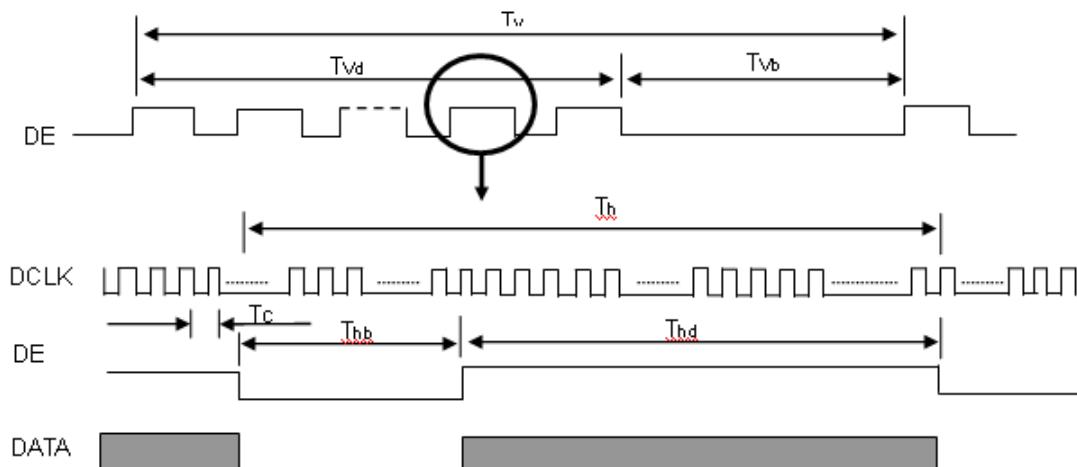
Note (1) The input clock cycle-to-cycle jitter is defined as below figures.  $T_{rcl} = |T_1 - T_1|$
