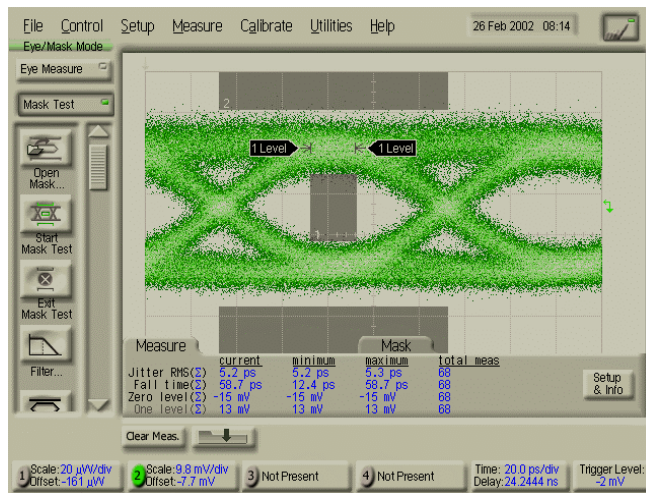
Figure 8. RA192 Eye Pattern at -26.2 dBm Input Power
