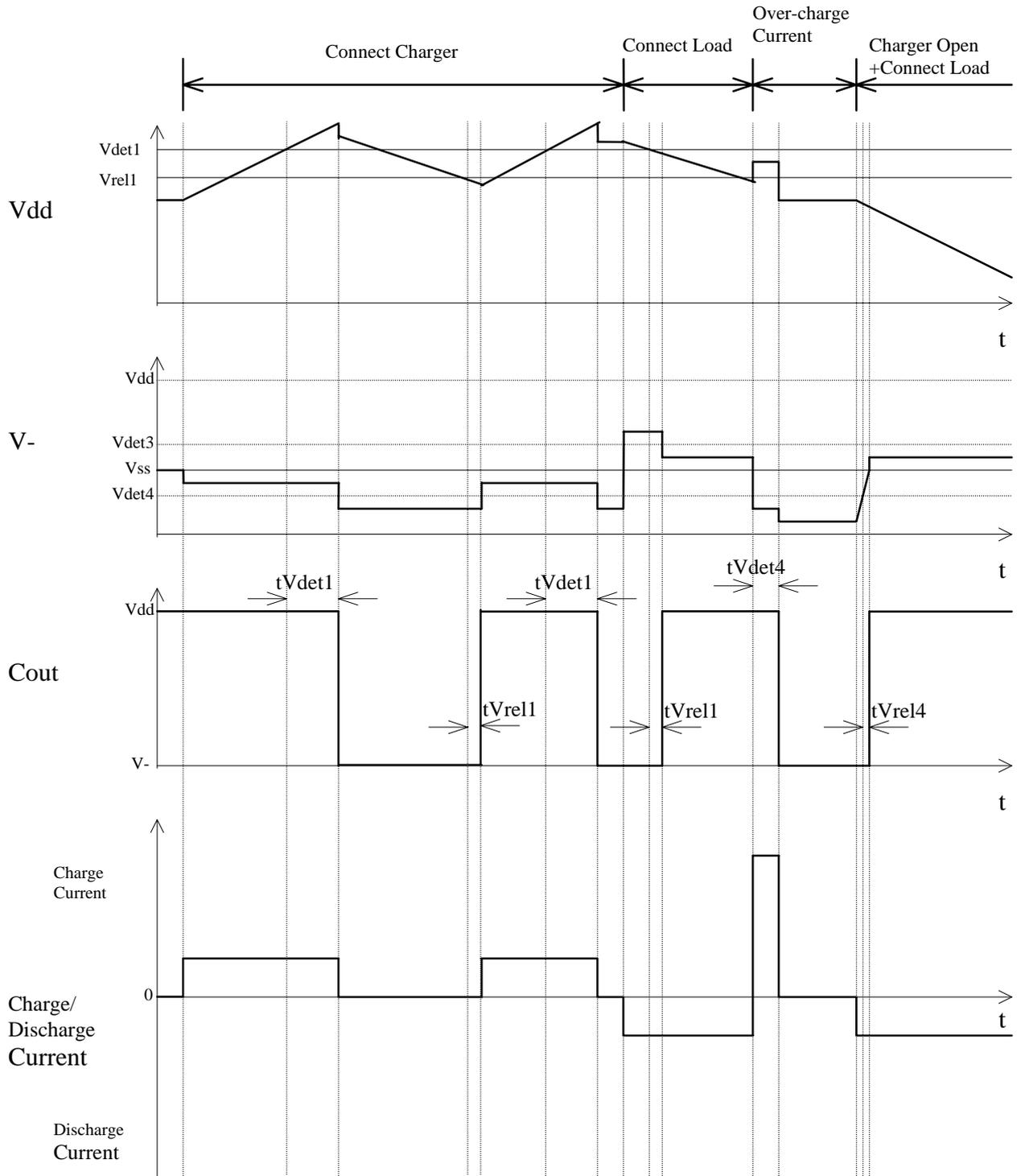
(2) Over-discharge, Excess discharge current, Short circuit
