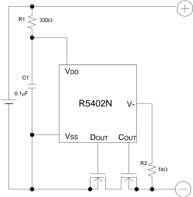
\*R1 and C1 stabilize a supply voltage to the R5402. A recommended R1 value is equal or less than 1kΩ. A large value of R1 makes detection voltage shift higher because of the conduction current flow in the R5402.
