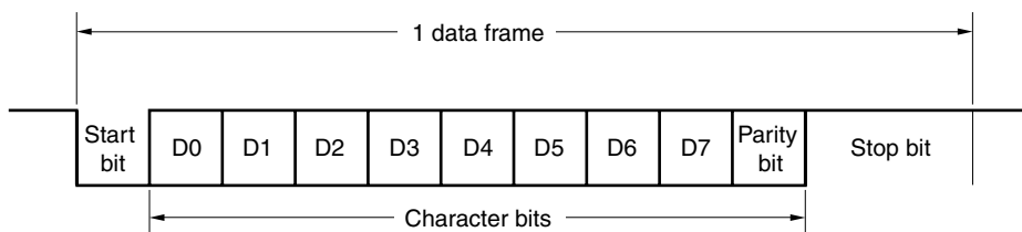
Figure 12-6. Format of Normal UART Transmit/Receive Data
