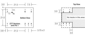
It is recommended to additionally bond the /277 version of the converter to the PCB if the application is subject to vibration or mechanical shock.
