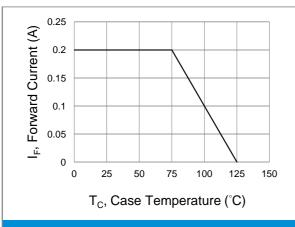
Fig.1 Forward Current Derating Curve
