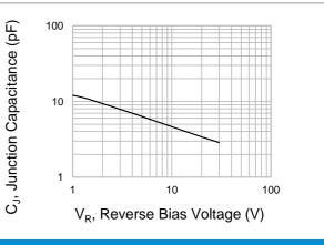
Fig.2 Typical Junction Capacitance
