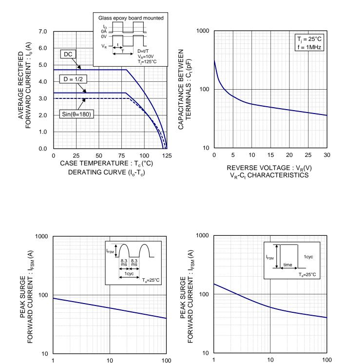
NUMBER OF CYCLES I<sub>FSM</sub>-CYCLE CHARACTERISTICS
